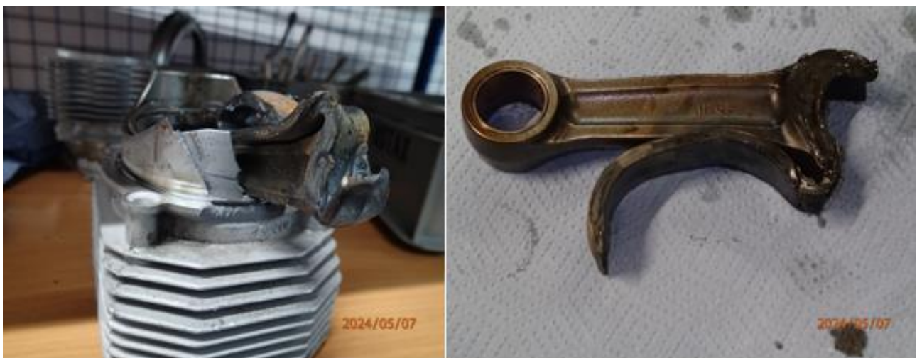
Figure 4: Connecting rod number three and two which had failed. Photo: Rotax/NSIA
