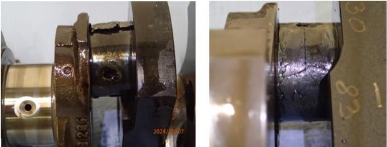
Figure 5: Close-up of connecting rod big end bearing three and two with clear signs of heat damage. Photo: Rotax/NSIA
