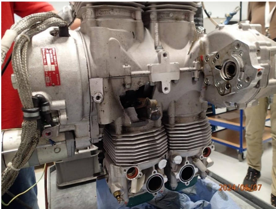
Figure 3: The connecting rod of cylinder number three which has punched through the crankcase. Photo: Rotax/NSIA
