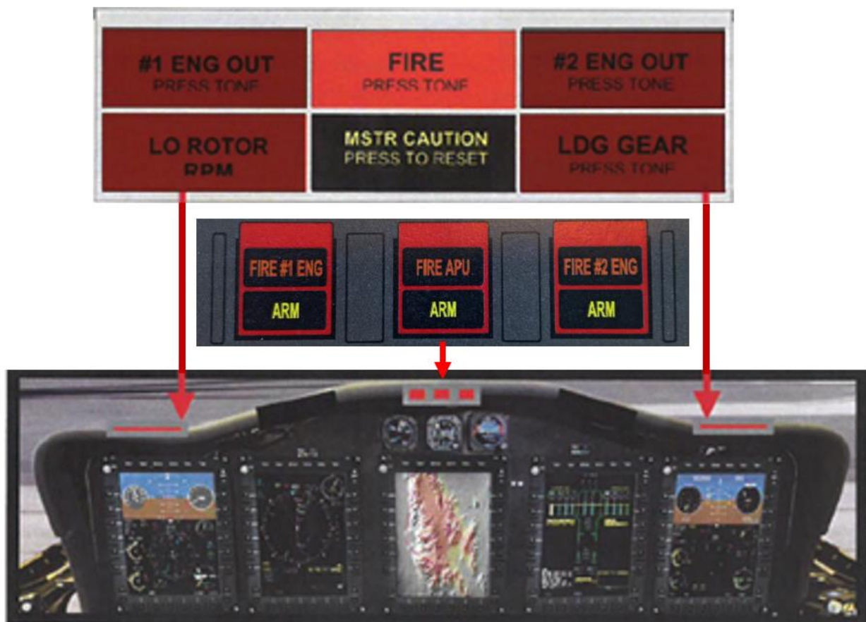
Figure 3: The warning light panels and their position in the cockpit. Source: Flight Safety International (Pilot Training Manual)/NSIA
