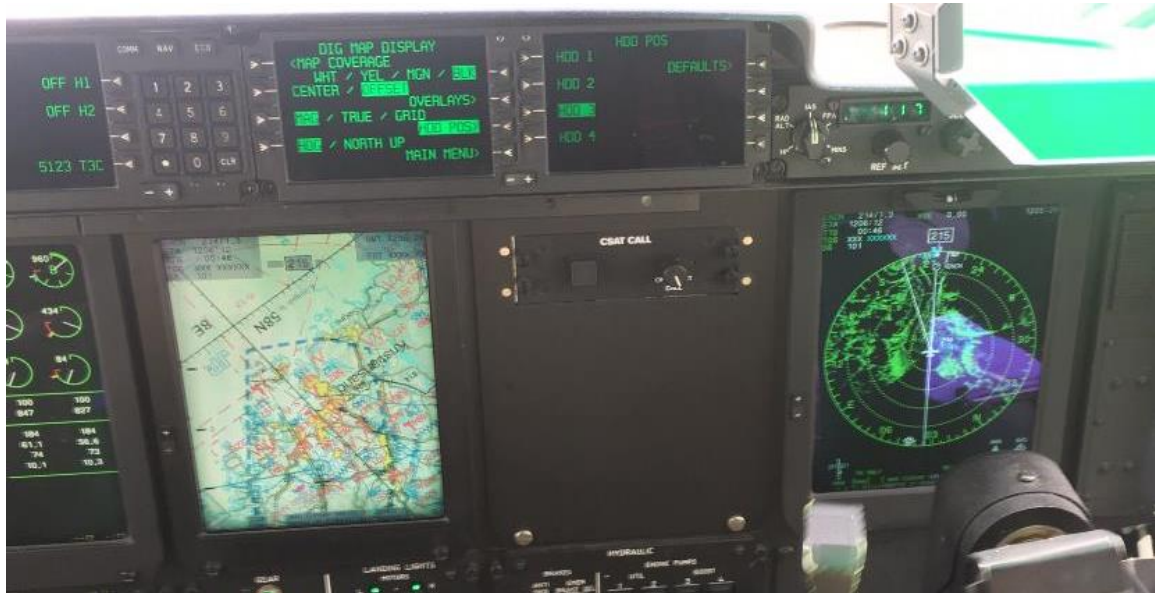
Figure 15: HDD 3 and HDD 4 on the right-hand side of the cockpit. HDD 3 displays a digital map while HDD 4 displays a monopulse ground map (MGM). Source: RNoAF
