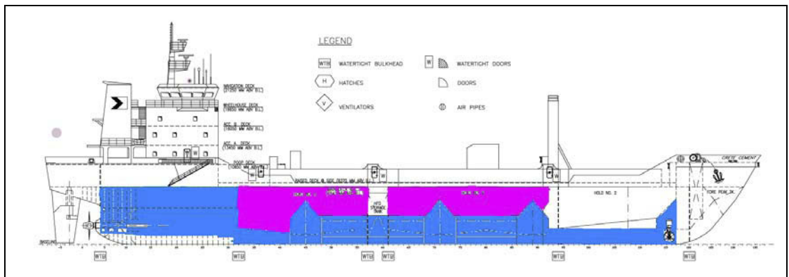
Figure 6: Flooding of vessel after running aground (scenario 2a).
