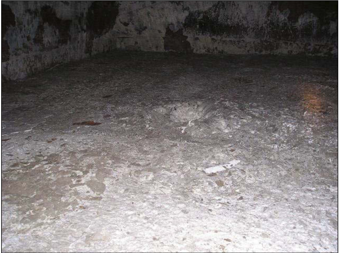
Figure 5: From cargo hold 3 after the water was pumped out and the cement had set. (Photo: DNV)
