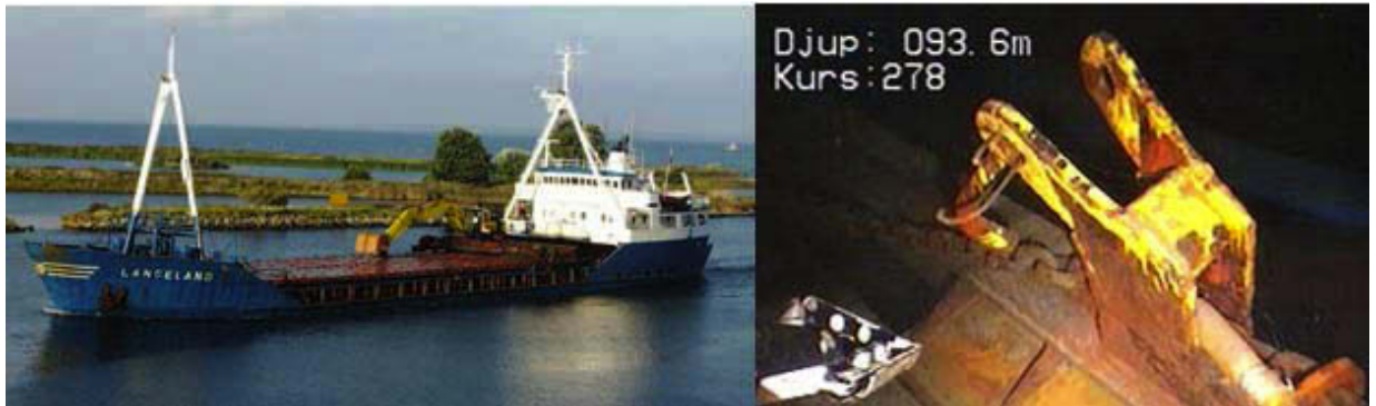
Figure 14: (Left) Excavator parked in normal position. (Right) One of two excavator attachments (starboard)
