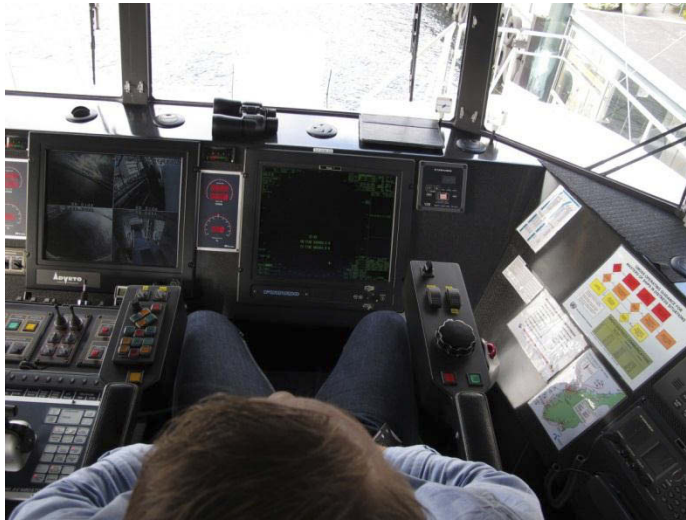
Figure 8: Illustration photo. Overview of the starboard navigator's seat. The armrest is fitted with a manual steering wheel and buttons for the takeover of control of manoeuvring. Photo: AIBN
