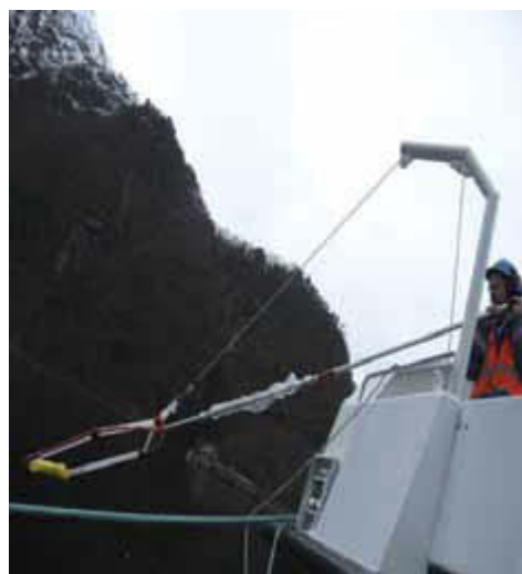
Figure 10: Photo of a rescue frame. The rescue sling (yellow and white line) lies flush with the frame. The line from the rescue sling runs through the pulley to the davit. Photo: Norled AS
