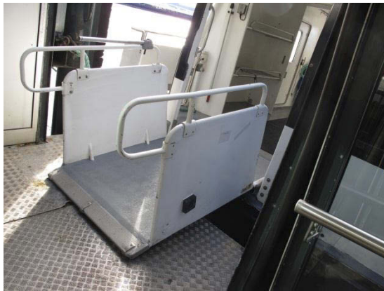
Figure 4: Gangway on the starboard side of the aft deck, seen from the quay. The gangway rests on the quay's surface. The black block on the side of the gangway is there to secure the gangway when in the vertical position. Photo: AIBN.
