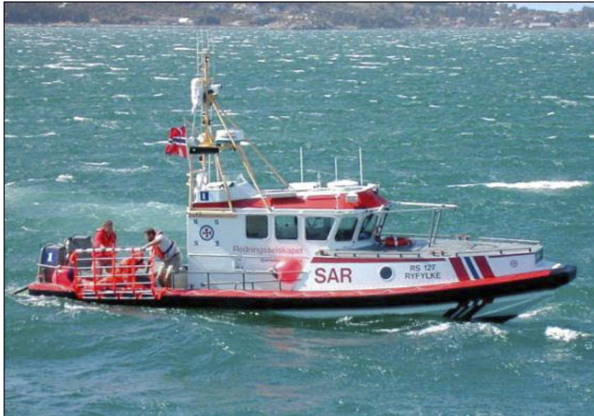
Figure 15: SAR vessel with a Dacon rescue net. These are used on board SAR vessels with low freeboard. Source: the Norwegian Society for Sea Rescue.
