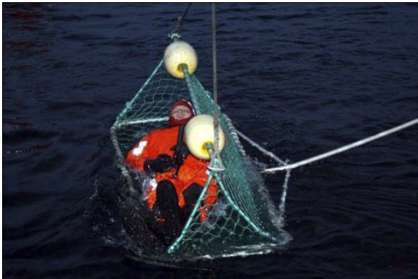
Figure 13: Måløy rescue cages with cranes have been installed on the large SAR vessels. The rescue cage is effective and simple to use, and recovery is quick. It can be used up to moderate weather conditions. Source: the Norwegian Society for Sea Rescue.
