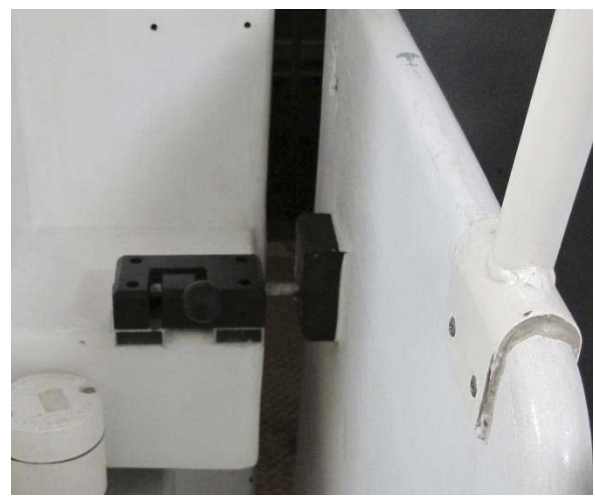
Figure 7: The locking bolt for the starboard gangway on the aft deck is secured. Photo: AIBN.
