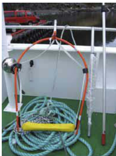
Figure 10: Photo of a rescue frame. The rescue sling (yellow and white line) lies flush with the frame. The line from the rescue sling runs through the pulley to the davit. Photo: Norled AS
