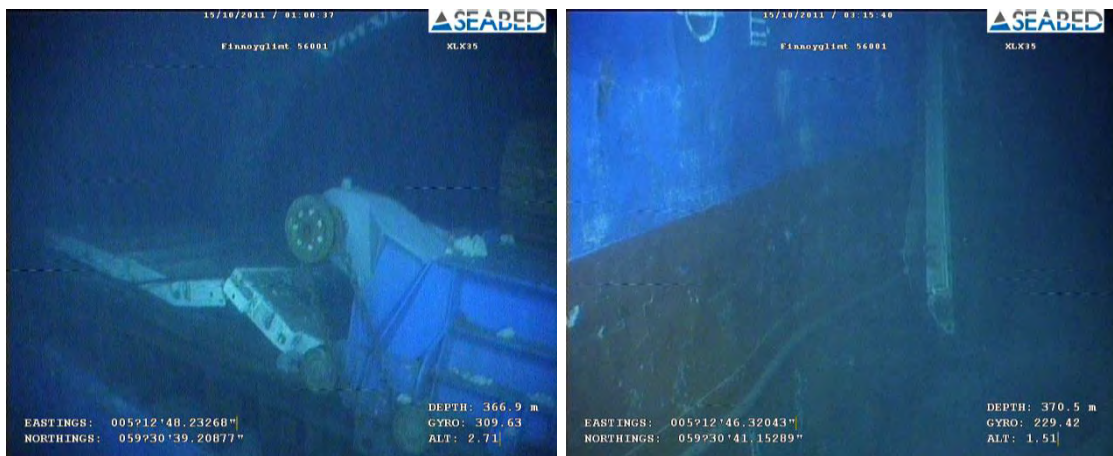
Figure 7: The photo on the left shows hatch cover no 6 bent upwards at the aft end and hatch cover no 7 bent upwards at the forward end. The photo on the right shows a cargo hatch cover that lay on Finnøyglimt's starboard side, fastened with a wire. Source: Seabed Worker's ROV
