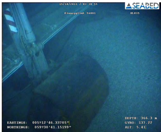
Figure 11: The photo shows the excavator bucket and arm dug into the aggregate in the cargo hold. The photo also shows how the cargo in the hold has been thrown towards the port side. Source: Seabed Worker's ROV
