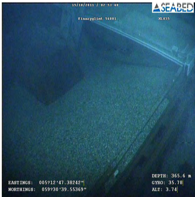
Figure 10: The photo shows how the cargo has been ‘thrown’ (shifted) towards the port side. Source: Seabed Worker’s ROV
