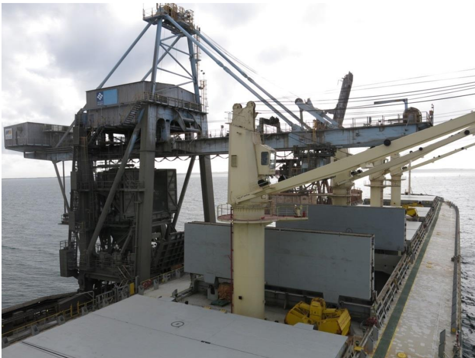
Figure 4: 'MV Favorita' is a handy-max bulk carrier with five cargo holds and four cargo handling cranes. Photo: AIBN
