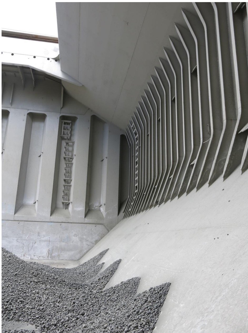
Figure 5: Shape of cargo hold 3 with a cargo of cement clinker. Photo: AIBN
