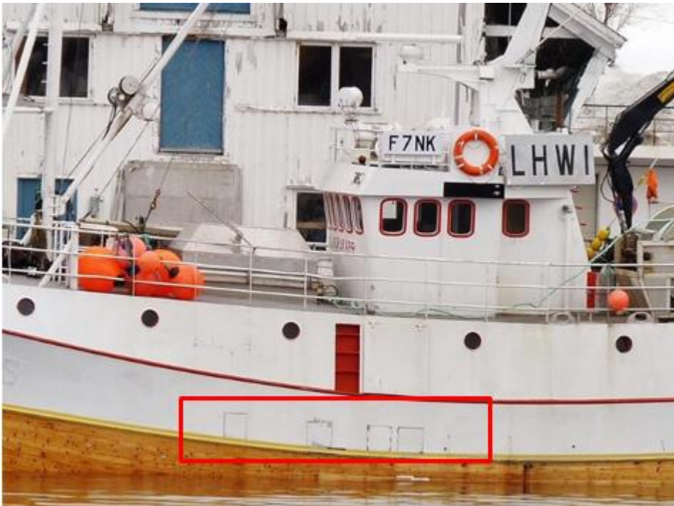
Figure 18: Photo of 'Østbanken' taken 11 April 2010 on which four freeing ports can be seen within the rectangle marked by the red lines. Photo: Roar Jensen
