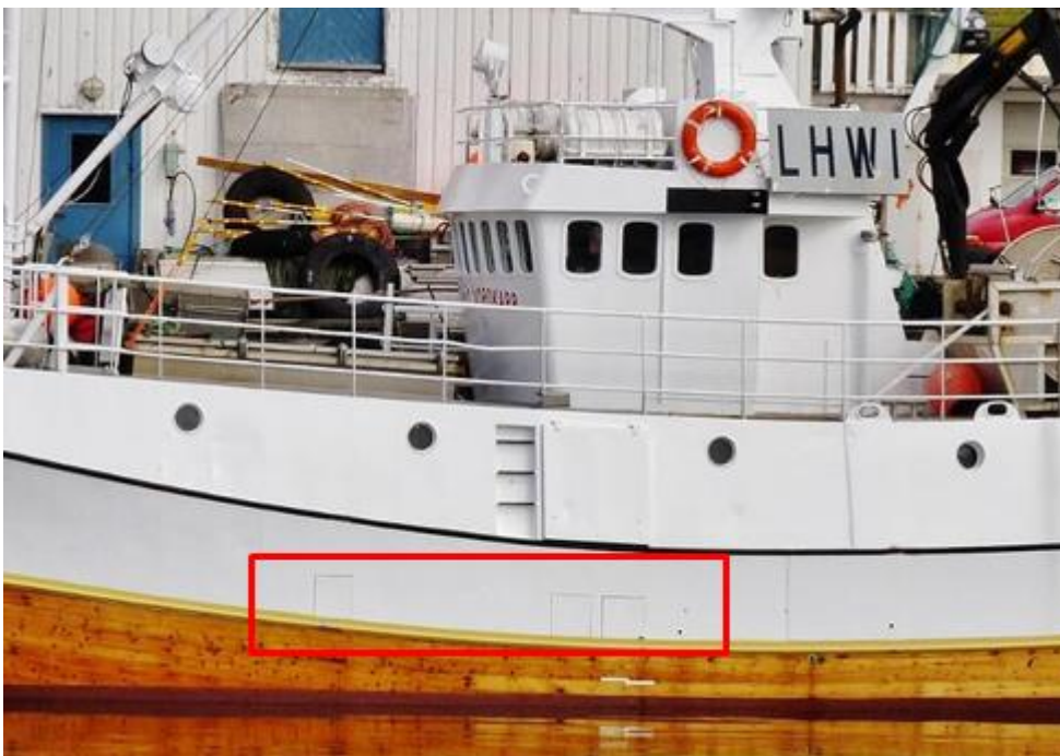
Figure 19: Photo of 'Østbanken' taken 22 May 2011 on which three freeing ports can be seen within the rectangle marked by the red lines. Photo: Roar Jensen
