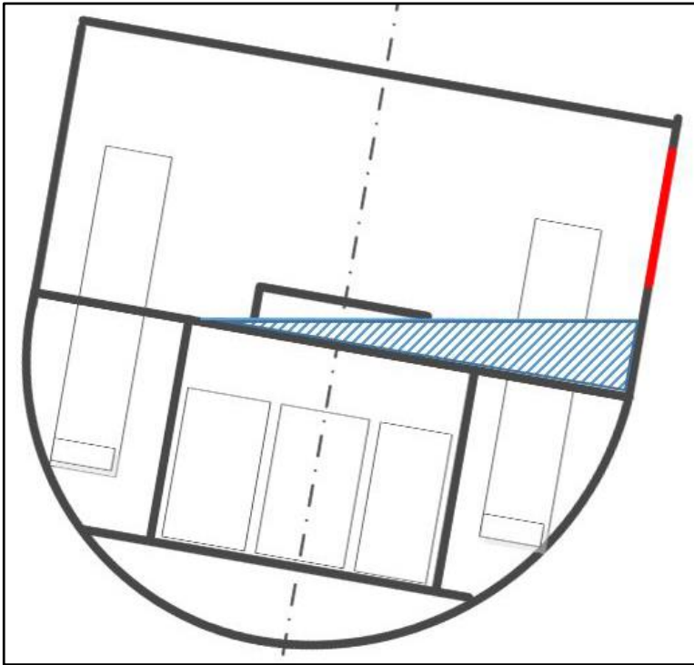
Figure 22: Simple schematic diagram of 'Østbanken' listing 10 degrees to starboard. The hatched blue area shows water on deck on the starboard side. Illustration: AIBN
