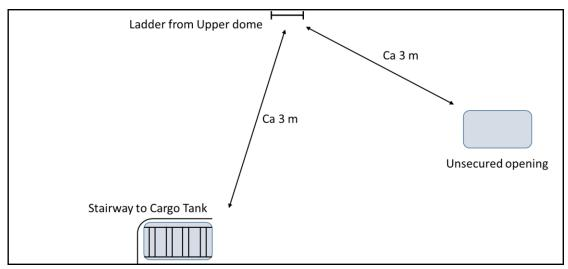
Figure 4: Schematic diagram of the deck in the lower dome. Illustration: AIBN
