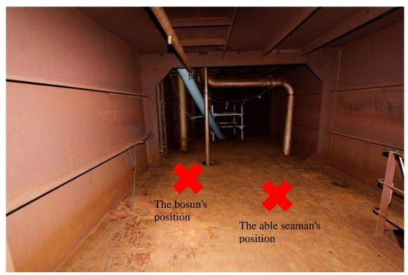
Figure 6: Photo from the lower dome. The unsecured opening can be seen at the far end. The guardrails were not in place at the time of the accident. The photo also shows the ventilation hose that had been fed into the tank through the unsecured open hatch. The red crosses indicate the approximate work positions of the bosun and able seaman. Photo: Asker and Bærum Police
