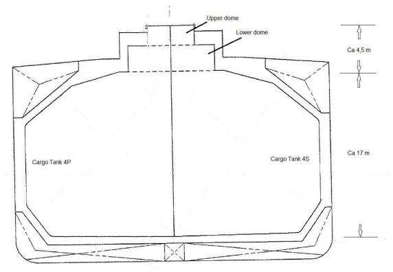
Figure 3: Schematic diagram of the vessel's cross-section at cargo tank no 4. Source: Drawing provided by BW Havfrost and edited by the AIBN
