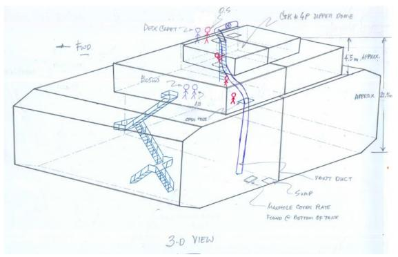
Figure 7: 3D drawing of cargo tanks 4S and 4P. The schematic diagram shows the positions and movements of the crew that were inside the tank at the time of the accident. Illustration: BW Havfrost
