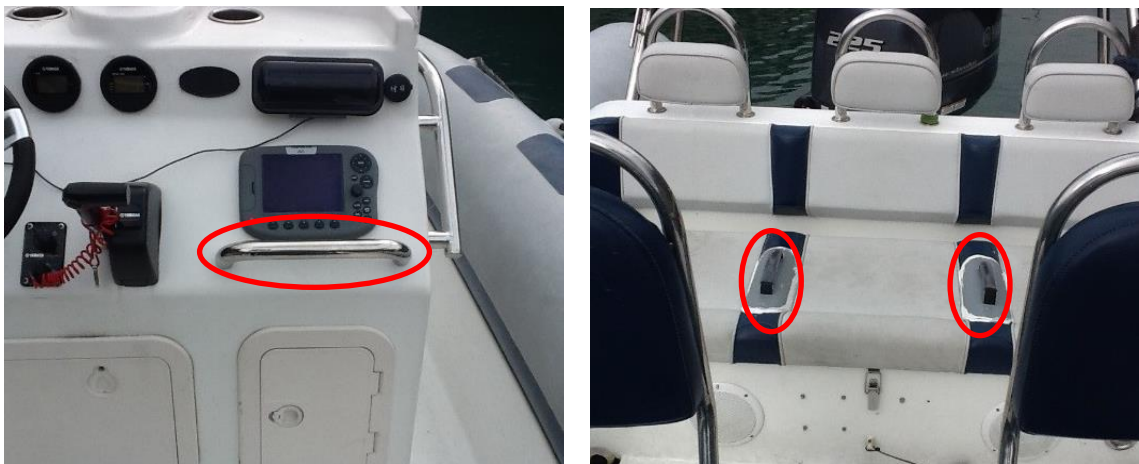
Figure 11: New handholds fitted after the accident. Photo: Briksdal Adventure
