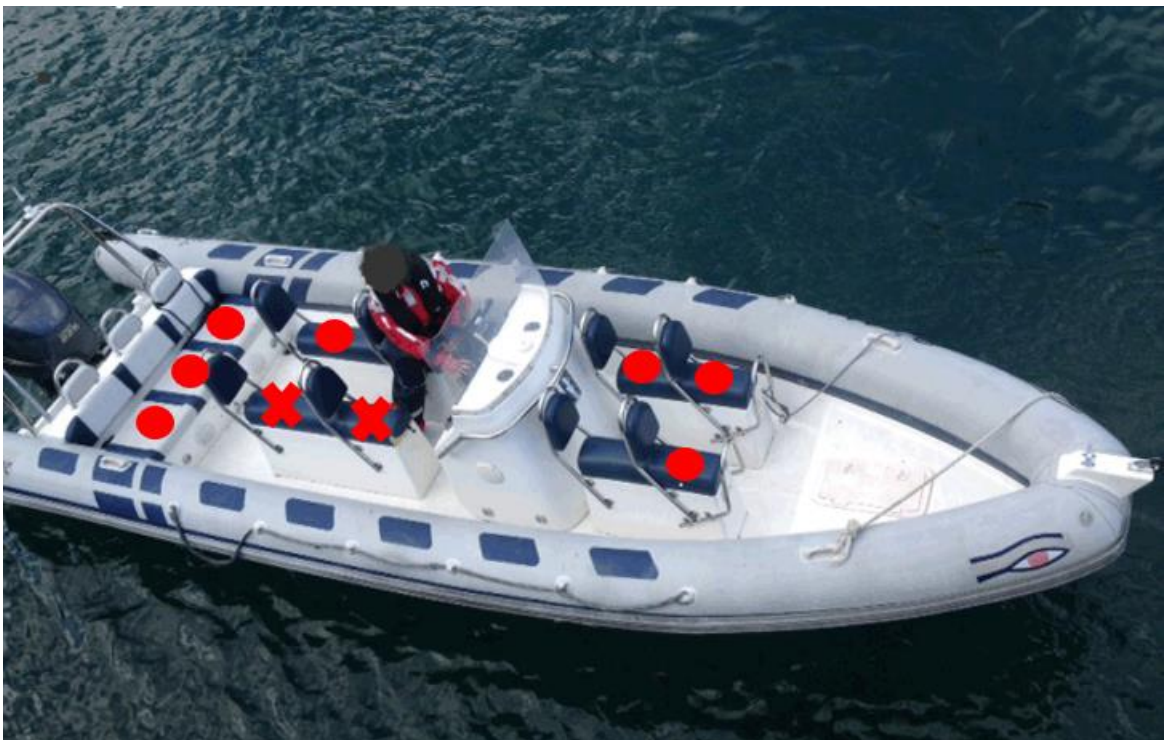
Figure 9: The RIB's seating configuration. The red circles mark where the passengers were sitting and the red crosses mark the passengers who fell into the water. Photo: AIBN
