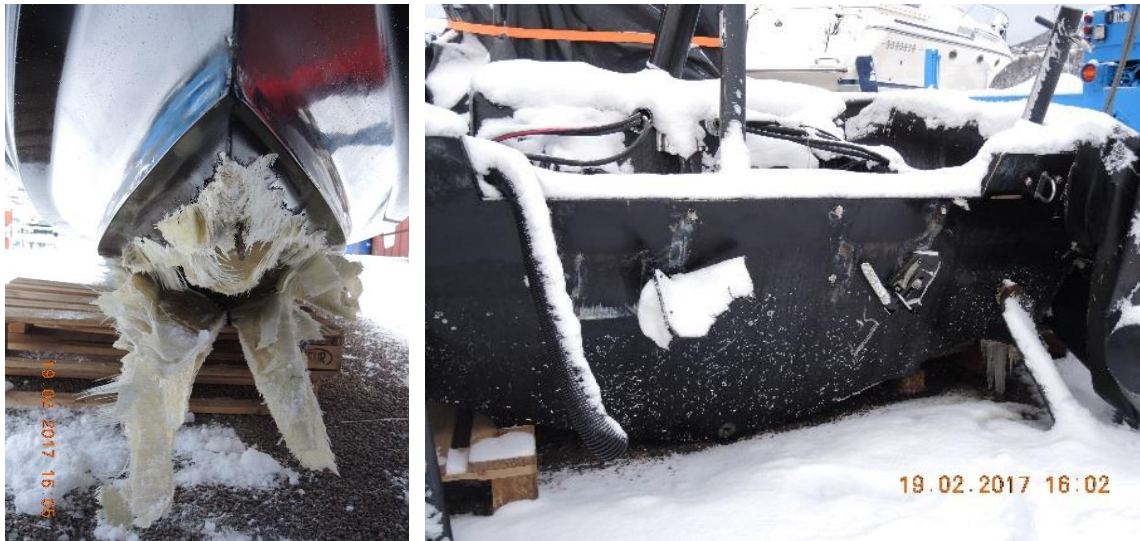
Figure 6: Damage to the bow (left) and damage to the stern (right). Photo: AIBN
