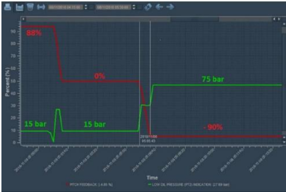
Figure 42: Change in pitch of port propeller, shown in IPMS. Screenshot: Navantia
