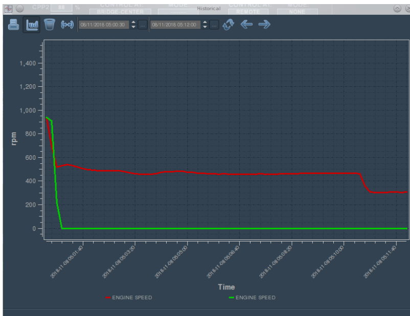
Figure 43: Speed curves for the starboard and port propulsion lines, shown in IPMS. Screenshot: The Navy/NSIA
