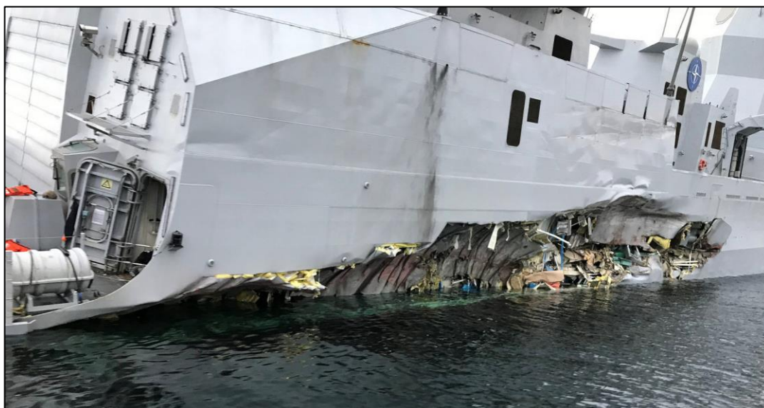
Figure 3: Damage along the frigate's starboard side following the collision. Photo: The Norwegian Coastal Administration
