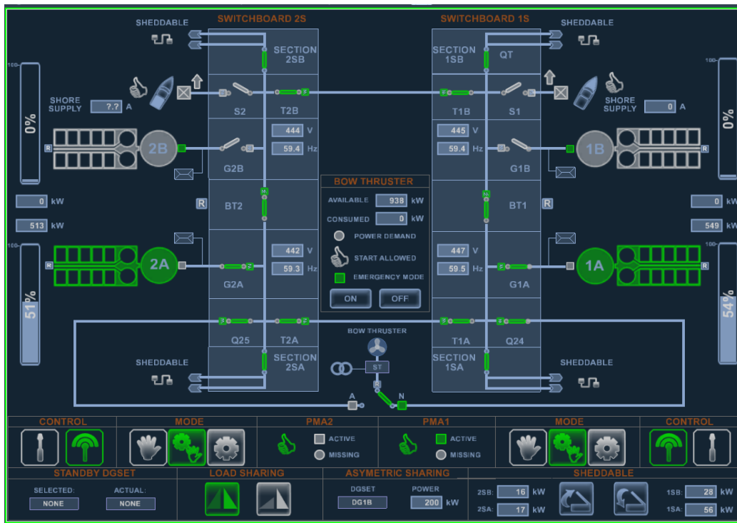
Figure 27: Power production status prior to the collision, shown in IPMS. Screenshot: NSIA
