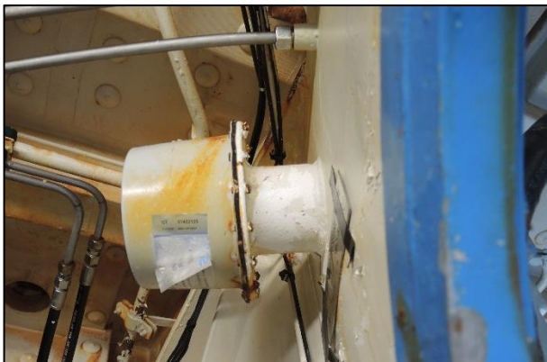
Figure 51: Spring-loaded over pressure valve. Photo: NSIA
