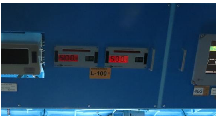
Figure 30: Rudder angle indicators showing starboard and port rudder angle, respectively. Photo: NSIA (from HNoMS ‘Thor Heyerdahl’)
