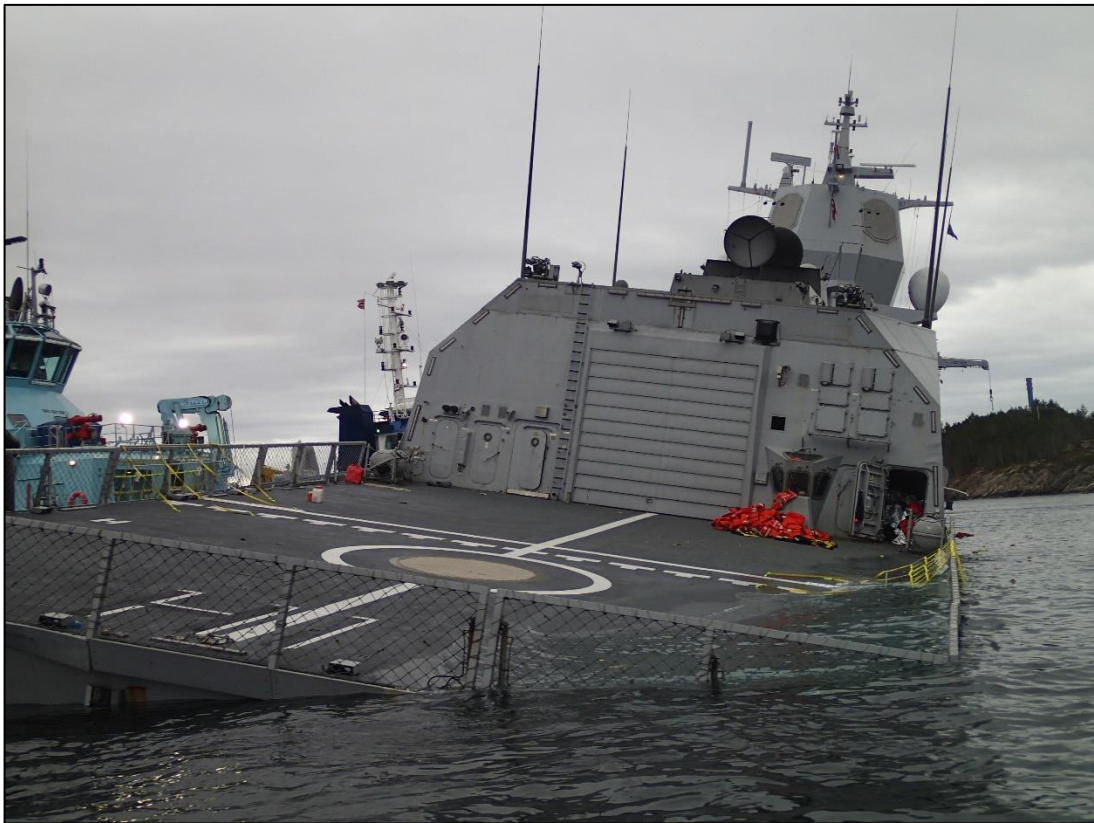
Figure 81: The helideck at HNoMS 'Helge Ingstad' under water on starboard side. Photo: CGV 'Bergen'
