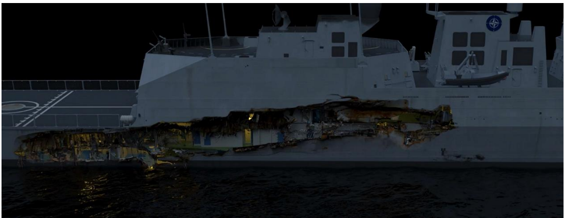
Figure 21: The damage on HNoMS 'Helge Ingstad'. Illustration: NCIS/CIAAS/NSIA
