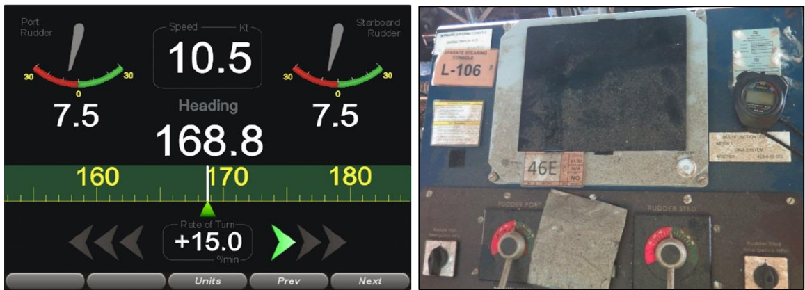
Figure 31: On the left: MFD showing speed, heading and rudder angle. On the right: Photo taken on HNoMS 'Helge Ingstad' after it was refloated. Showing SSC with tillers and MFD covered by Plexiglas, not to affect night vision negatively. Screenshot: The Navy. Photo: NSIA
