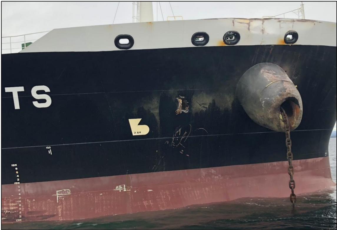
Figure 4: The hawsepipe and the damage sustained by 'Sola TS'. Photo: The Norwegian Maritime Authority
