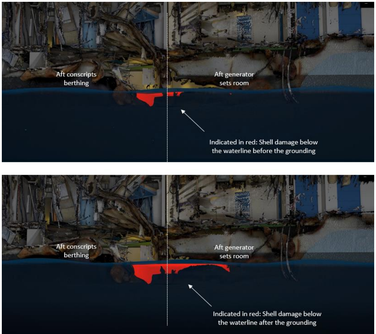
Figure 68: Shell damage relative to the waterline before and after grounding. Illustration: NCIS/CIAAS/NSIA
