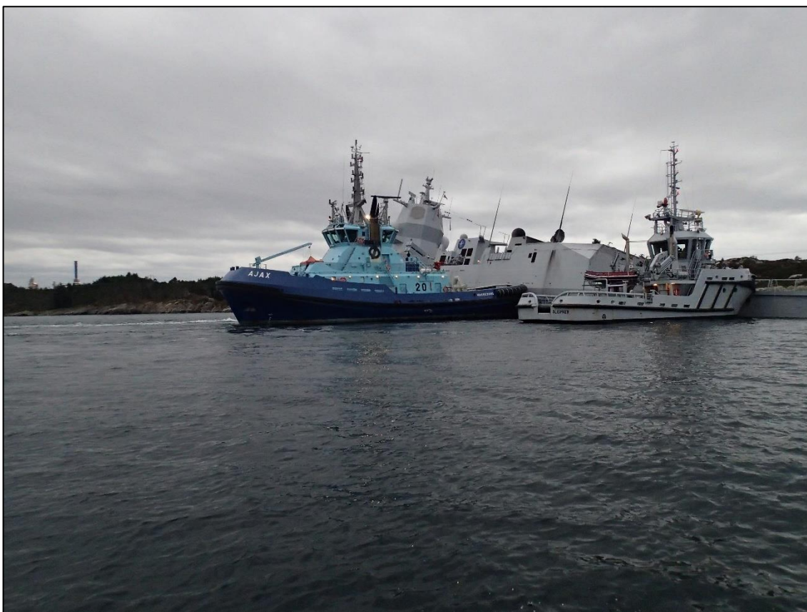
Figure 15: Tugs pushing HNoMS 'Helge Ingstad' towards shore. Photo: CGV 'Bergen'
