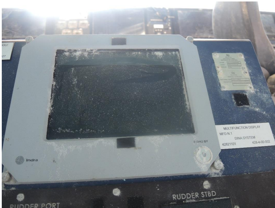
Figure 1: MFD9 in front of the helmsman on SSC. The photo was taken after the refloating of HNoMS 'Helge Ingstad', with the cover on the display removed. Photo: NSIA
