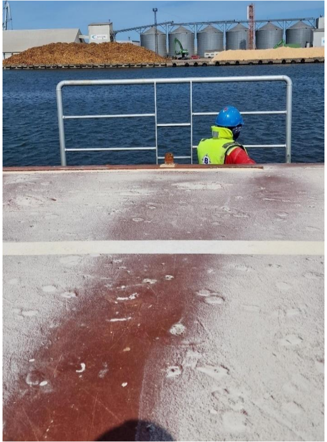
Figure 15: Higher railings installed locally on similar vessel (seen from the hatch deck). Photo: Berge Rederi AS
