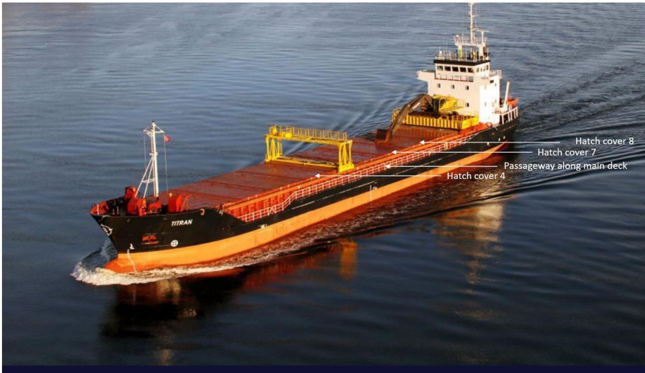
Figure 3: Passageway along the main deck and cargo hatches. Photo: Berge Rederi AS. Illustration: The NSIA
