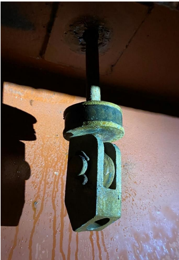
Figure 9: Cleat placed under the rail track to secure the cargo hatches to the coaming. Photo: NSIA
