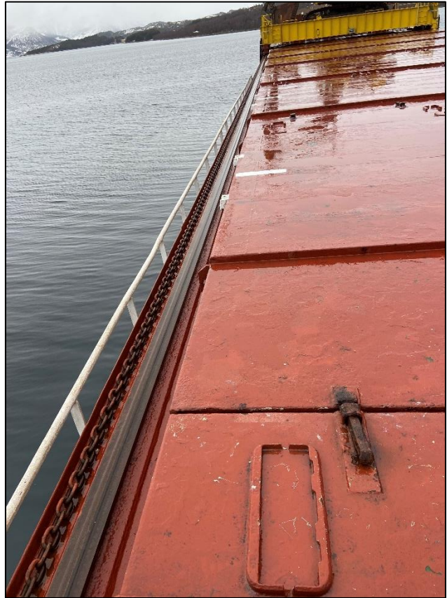
Figure 5: Rail track along the cargo hatches. Photo: NSIA
