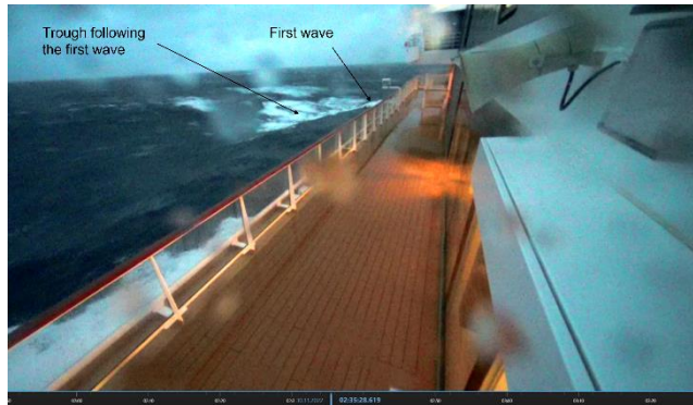
Figure 7: The first wave hitting the side of the ship. White foam is visible in the trough that follows at 22:35:28. Source: CCTV
