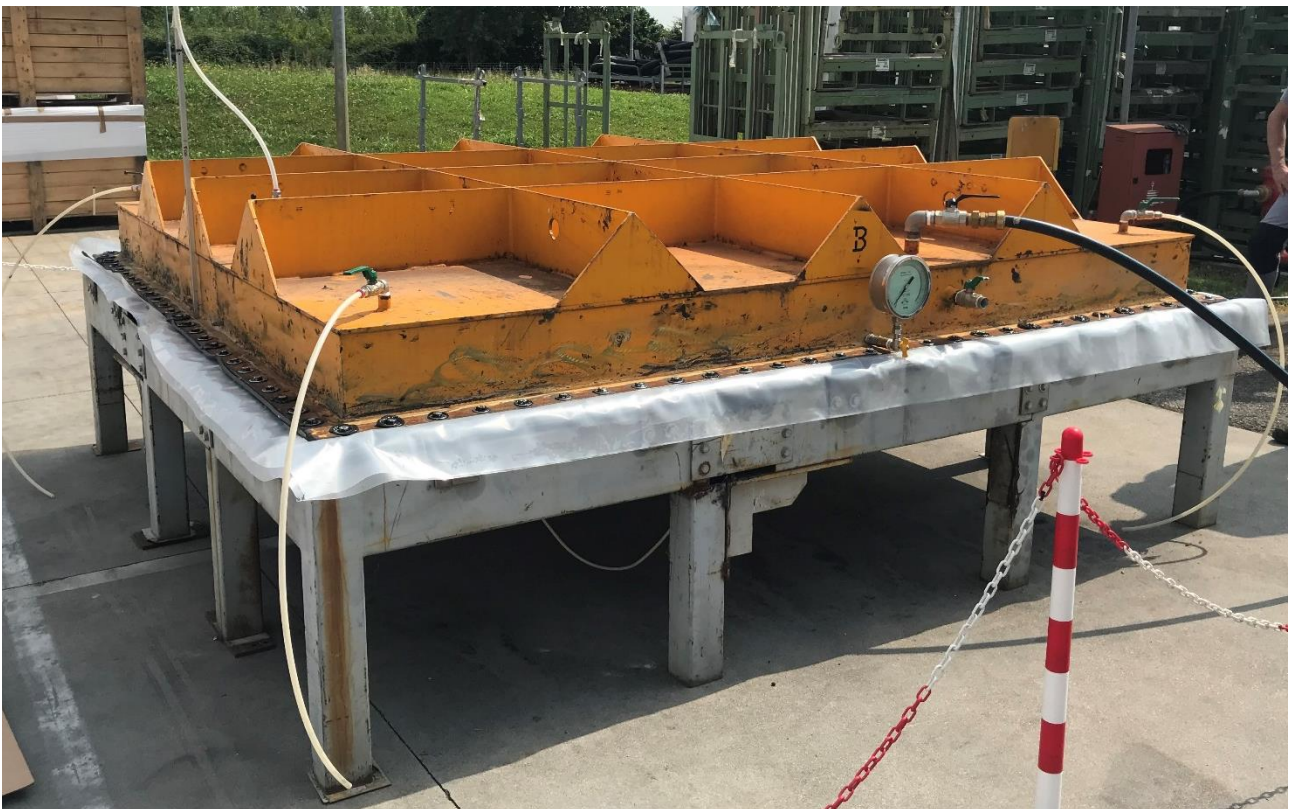
Figure 78: The hydrostatic test bench used in the full-scale test. Photo: Window supplier
