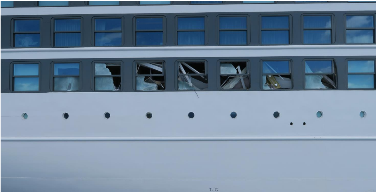
Figure 18: Damage to windows and frames in the damaged area on deck 2. Photo: NSIA
