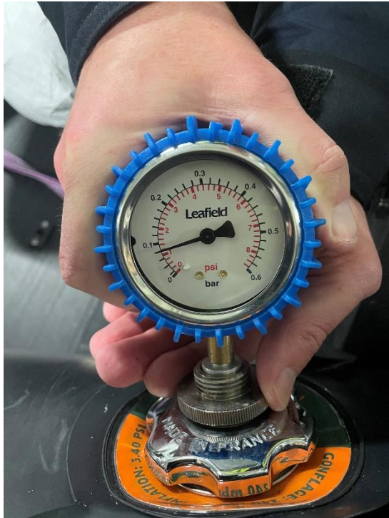
Figure 65: Manometer fitted to inflation valve. Photo: NSIA
