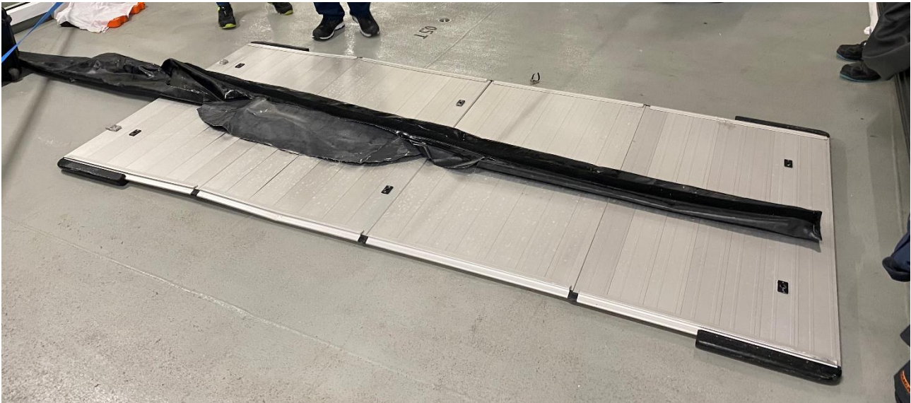
Figure 42: The centre keel stretched out on the floorboards in the position it was in during the incident. Photo: NSIA
