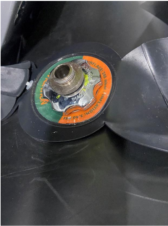
Figure 64: Inflation valve with overpressure relief. Photo: NSIA
