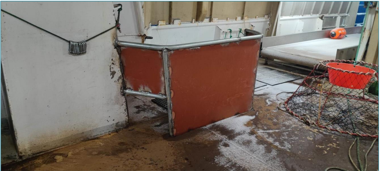
Figure 11: Steel barrier on the afterdeck to prevent falling overboard. Photo: Shipping company
