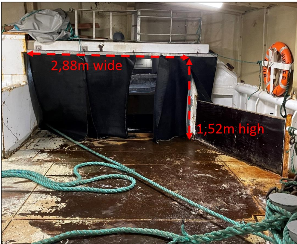
Figure 8: Setting hatch on aft working deck. Photo: NSIA
