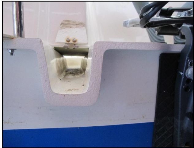
Figure 20: Port side drain opening from the Viking 7 investigation. Photo: NSIA
