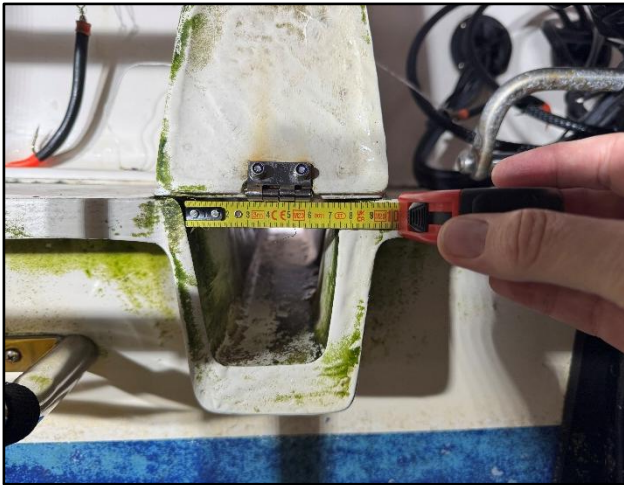
Figure 19: Port side drain opening on the accident vessel. Photo: NSIA
