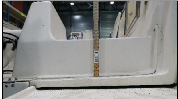
Figure 22: Recessed step on the starboard aft side, 12.5 cm above the deck. Photo: NSIA
