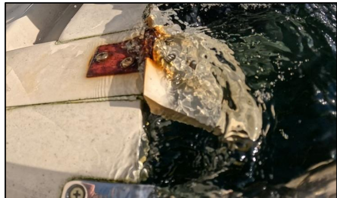
Figure 26: Port drain opening in open position as a result of aft trim in a wave trough. Photo: NSIA
