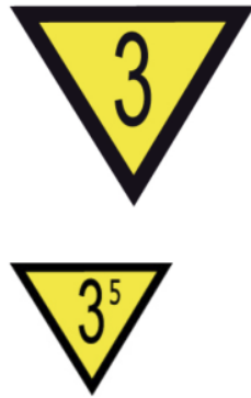
Figure 16: Signal 68 A 'Reduced speed' (the example shows 30 and 35 km/h) (source: the NNRA).
