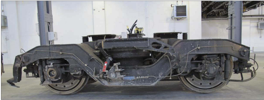
Figure 23: Leading bogie (photo: the AIBN).
