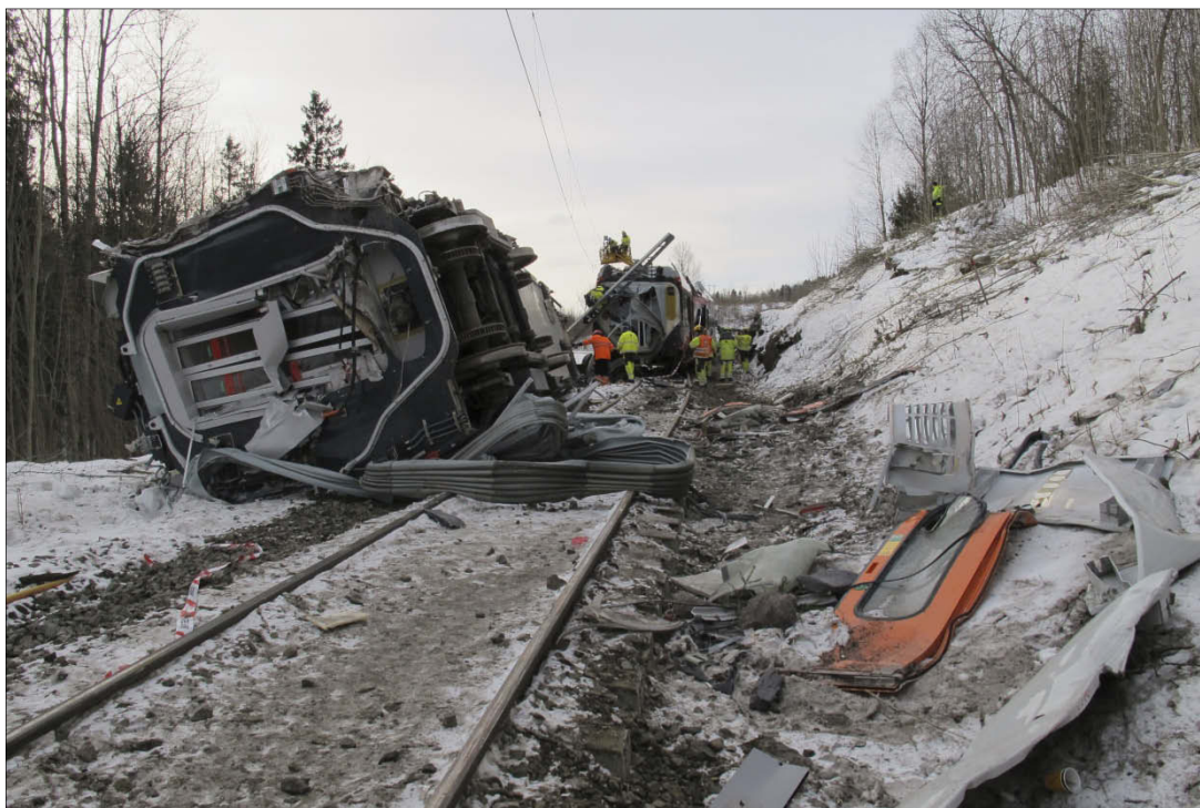
Figure 7: Carriage rolled on its side (photo: AIBN).
