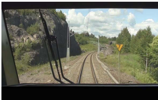
Figure 18: The speed signal for 70 km/h (photo: the AIBN).
