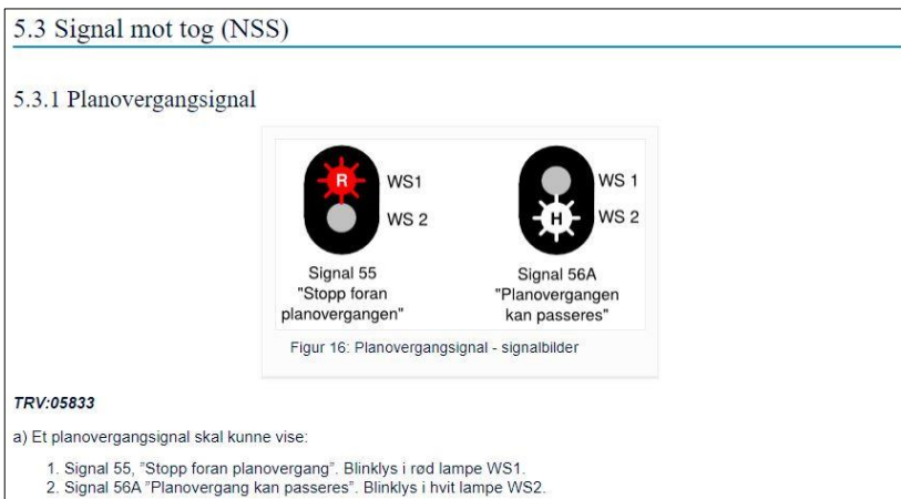
Figur 7: Planovergangssignal. Kilde: Bane NOR 3
