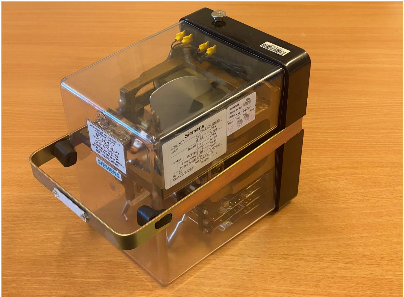
Figure 2: VT1-6F-4B relay. Photo: NSIA
