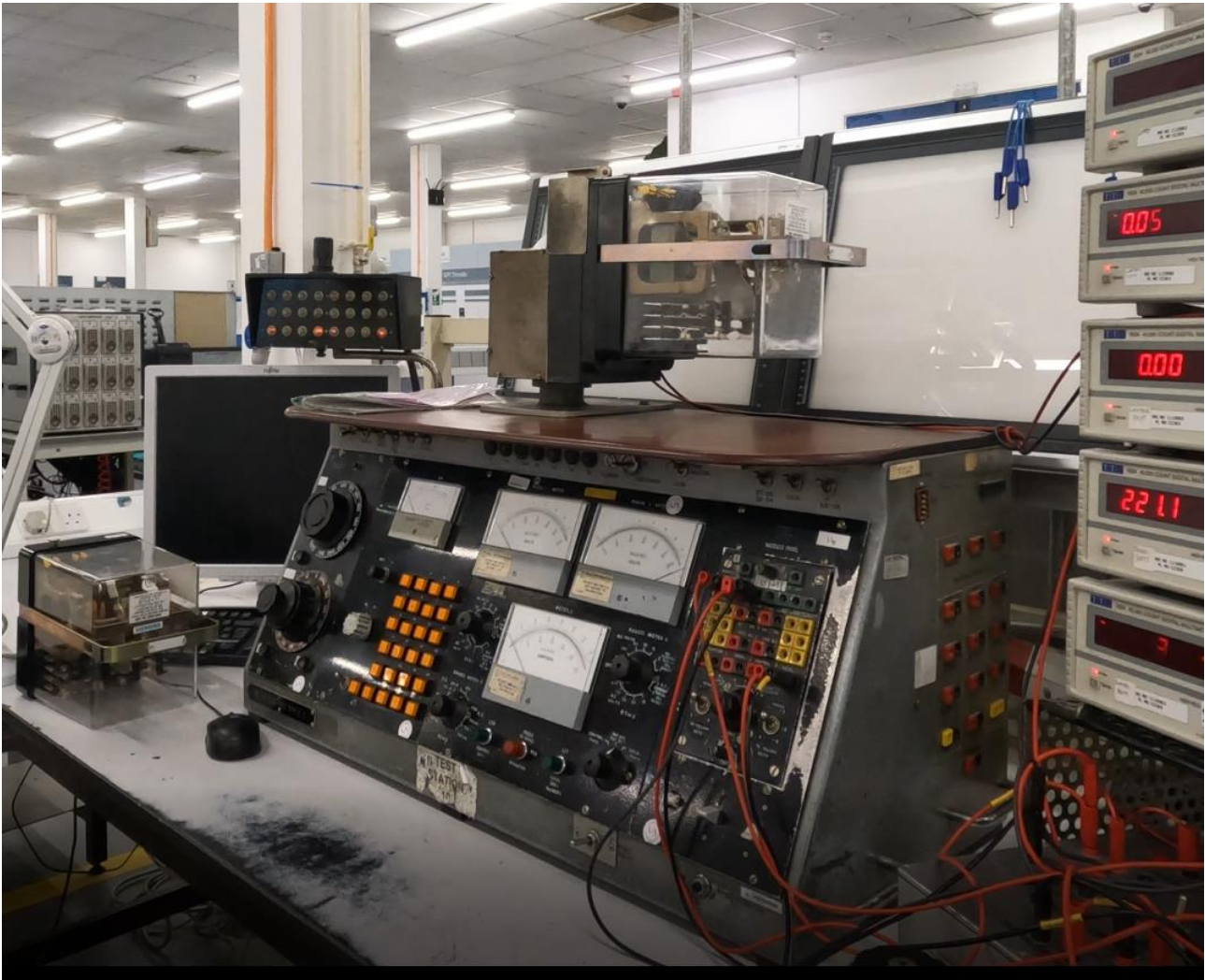
Figure 4: Comparable relay mounted on top of test bench. The relay involved in the incident can be seen on the left-hand side of the worktop. Photo: NSIA
