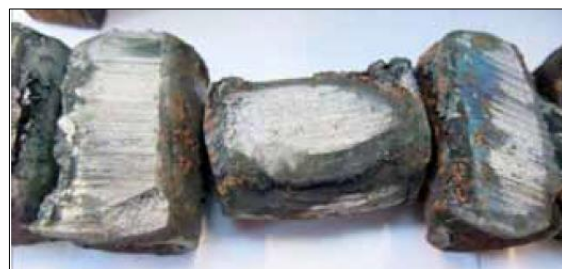
Figur 40: Eksempel tverrstilt rulle. Kilde: The Dutch Safety Board 7
