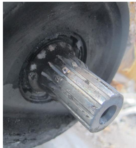
Figure 21: Worn drive shaft splines. Photo: AIBN
