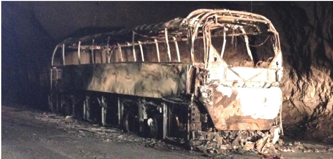
Figure 5: The burnt-out coach inside the tunnel. Photo: AIBN
