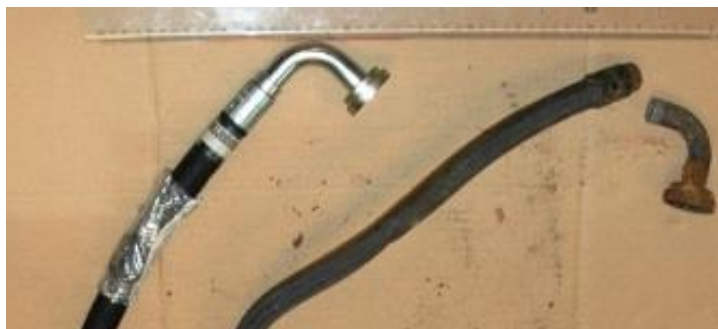
Figure 17: For reference purposes, the photo shows a new hydraulic hose on the left. The burnt-out and broken hydraulic hose is shown on the right. Photo: FOLAT
