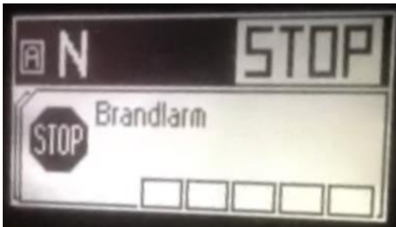
Figure 11: Dashboard display on release of the fire extinguishing system in a similar coach. Photo: Stenstorp Buss
