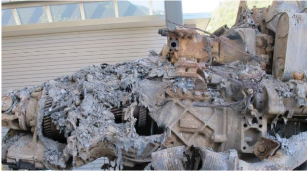
Figure 8: The damage to the coach's gearbox as a result of the fire. Photo: AIBN
