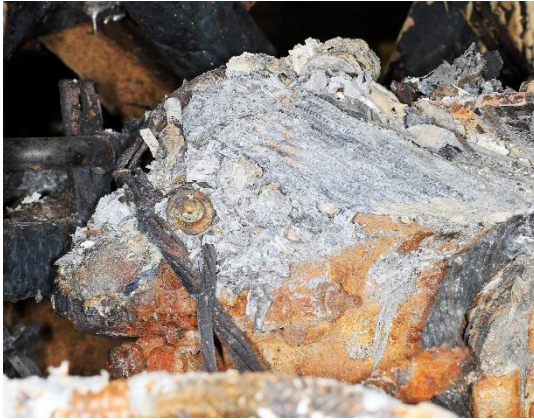
Figure 13: Hydraulic pump covered in melted aluminium after the fire. Photo: AIBN
