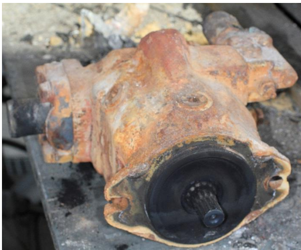
Figure 20: Disconnected hydraulic pump. Photo: AIBN
