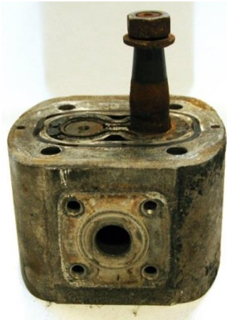
Figure 15: Fan motor for the cooling system. Photo: FOLAT
