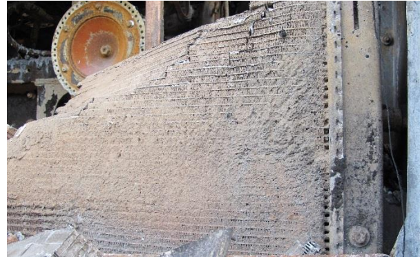
Figure 10: There were soil marks on the radiator. Photo: AIBN
