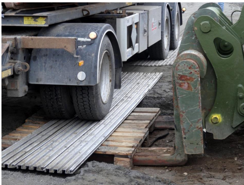
Photo 23. Lifting of the left front wheel of the trailer in order to simulate a turn over a bump between two lanes.
