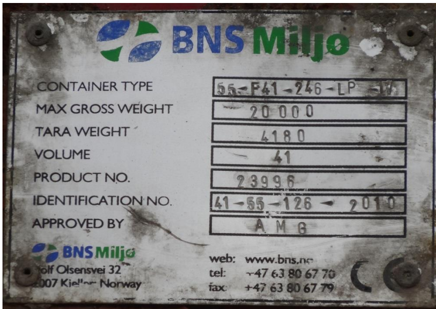
Photo 7. Marking of the hooklift container used on the truck.
