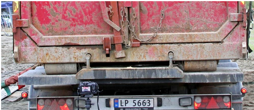
Photo 13. The trailer's two securing fittings at the aft end of the hooklift container.
