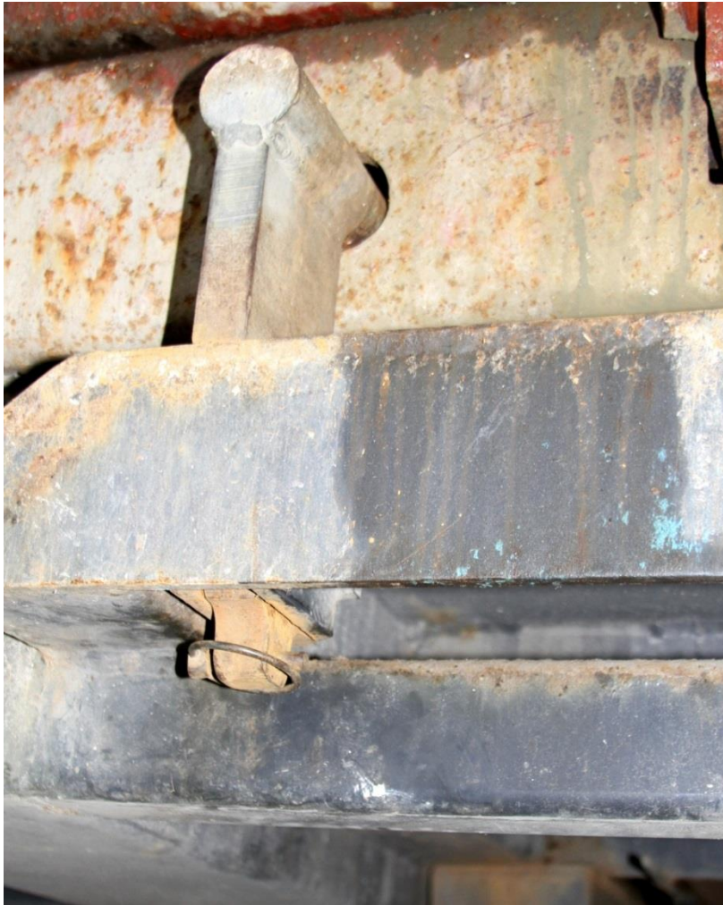
Photo 14. The aft fittings are secured by a pin prohibiting them from coming out. The pin is secured with an yoke.
