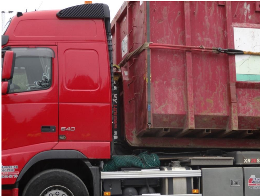
Photo 18. Force level equivalent to 0.5 g. The front part of the hooklift container has no contact with the load deck of the truck.
