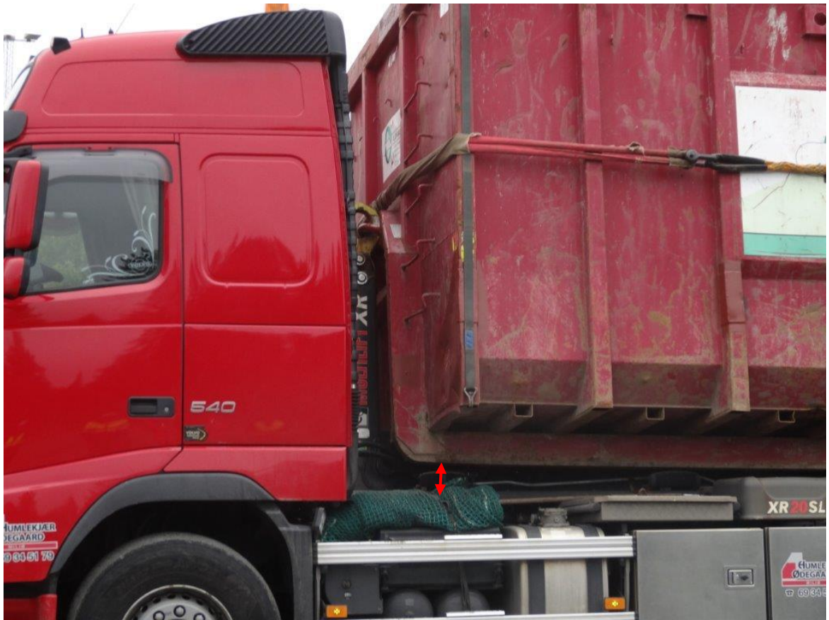
Figure 16: The hooklift container on the truck is lifted approximately 12 cm (see red arrow) at the front when exposed to a lateral load of approximately 0.5 G. Photo: SP
