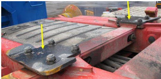
Figure 13: Retrofitted plates (black in colour, indicated by the yellow arrows) for mechanical locking of the container to the truck from the inside. The photo shows the plates installed as part of a JOAB hooklift system. Photo: AIBN
