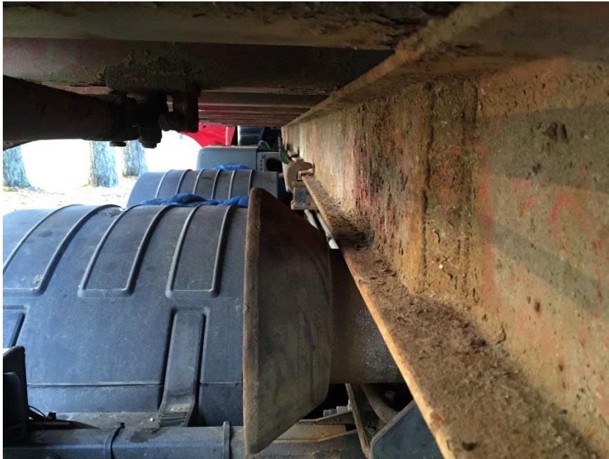
Photo 4. Part of the loading deck of the truck with the frame wheels which is supporting the container horizontally
