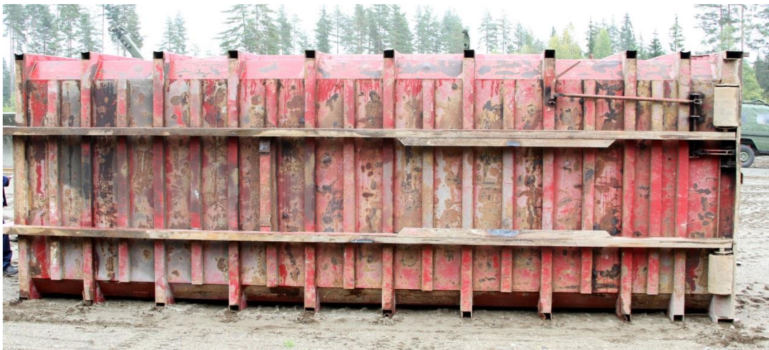
Photo 31. The hooklift container used on the trailer.
