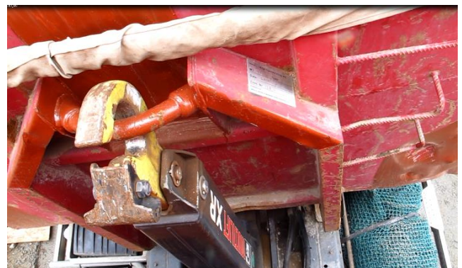
Figure 18: Hooklift arm and lift bar on container exposed to a lateral load of approximately 0.5 G. Photo: AIBN
