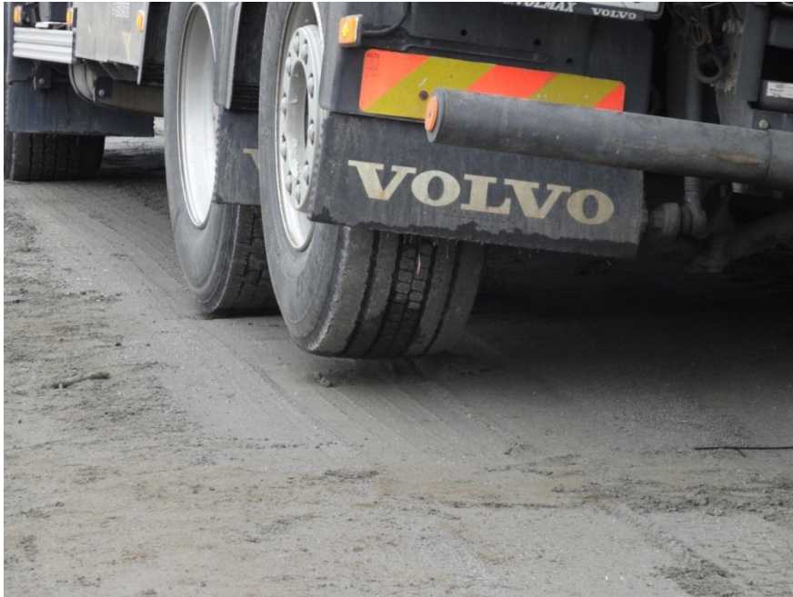
Photo 16. At a force level equivalent to 0.5 g were the aft wheels of the truck lifted from the ground.
