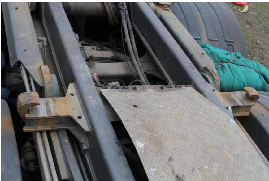
Photo 5. The two external securing hooks in the aft part of the loading deck.
