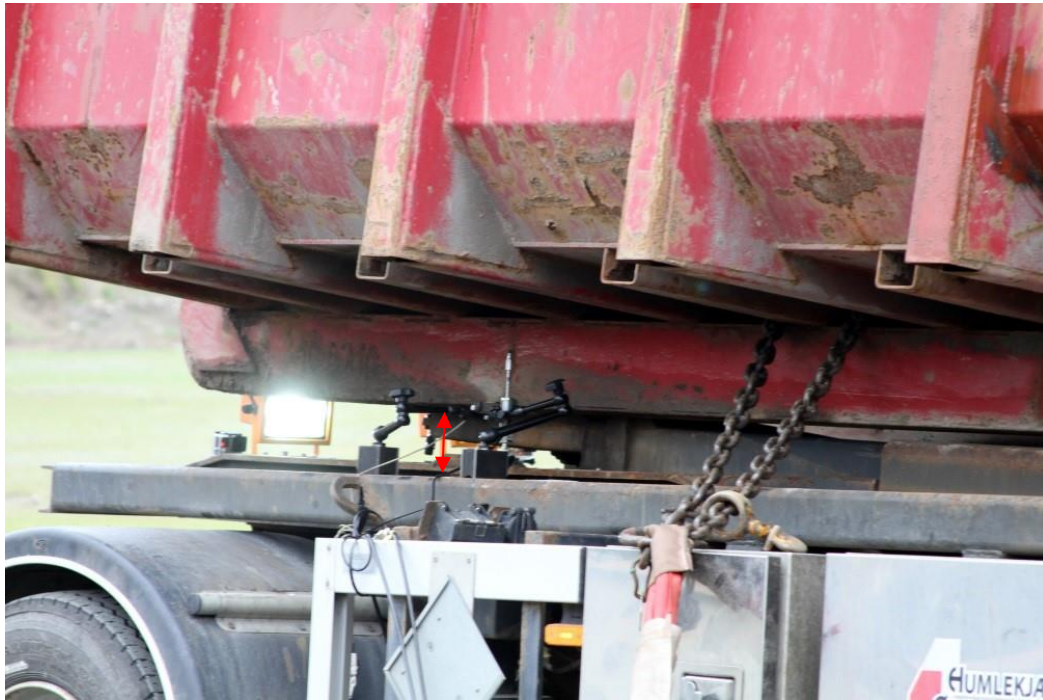
Figure 19: The front of the hooklift container is lifted more than 15 cm (see red arrow) when exposed to a lateral load of 0.38 G. Photo: SP
