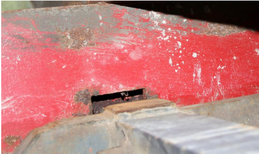
Photo 12. One of the securing devices fitted into the tilting frame of the trailer.
