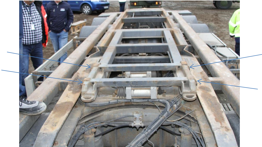
Photo 8. The load deck of the trailer, observe the four securing devices on the front part of the tilting frame.
