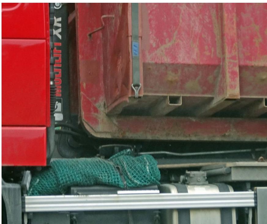
Photo 19. Detail from photo 18, the distance between container and load deck was estimated to 120 mm.
