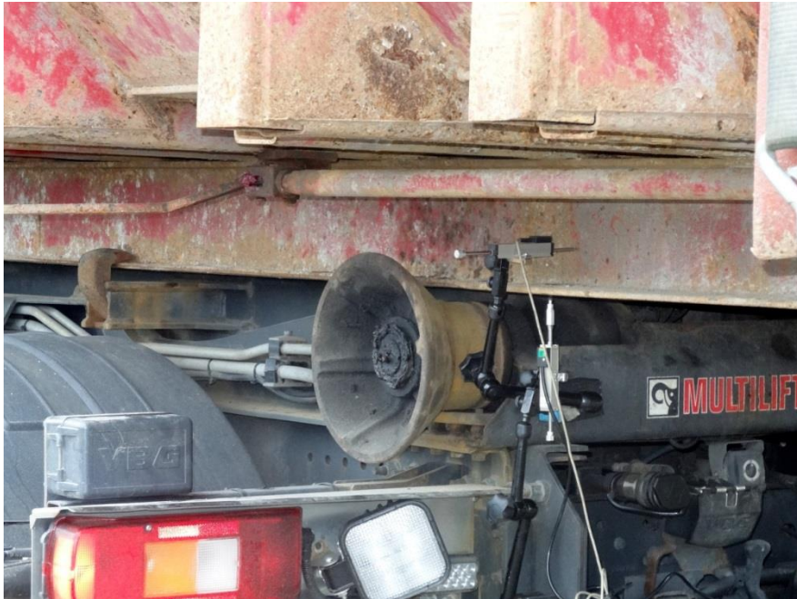
Photo 6. The indicators location when measuring movements between load deck and hooklift container in horizontal and vertical direction.
