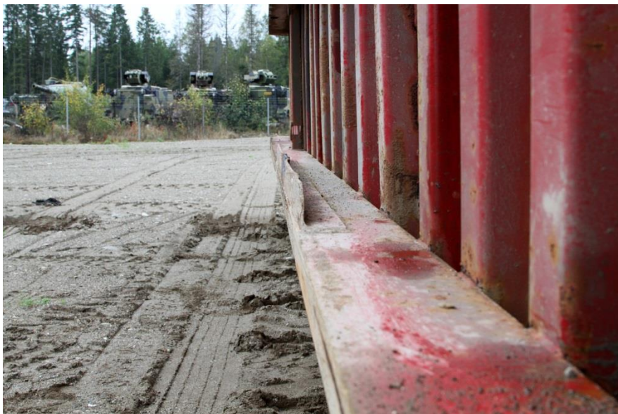
Photo 33. The container used on the trailer showed many traces from hard treatment and hasty repairs.
