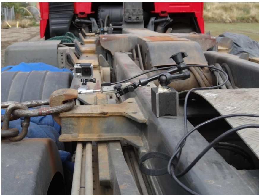
Photo 26. Position of indicator for measuring of the movements of the locking hooks on the left side of the truck.
