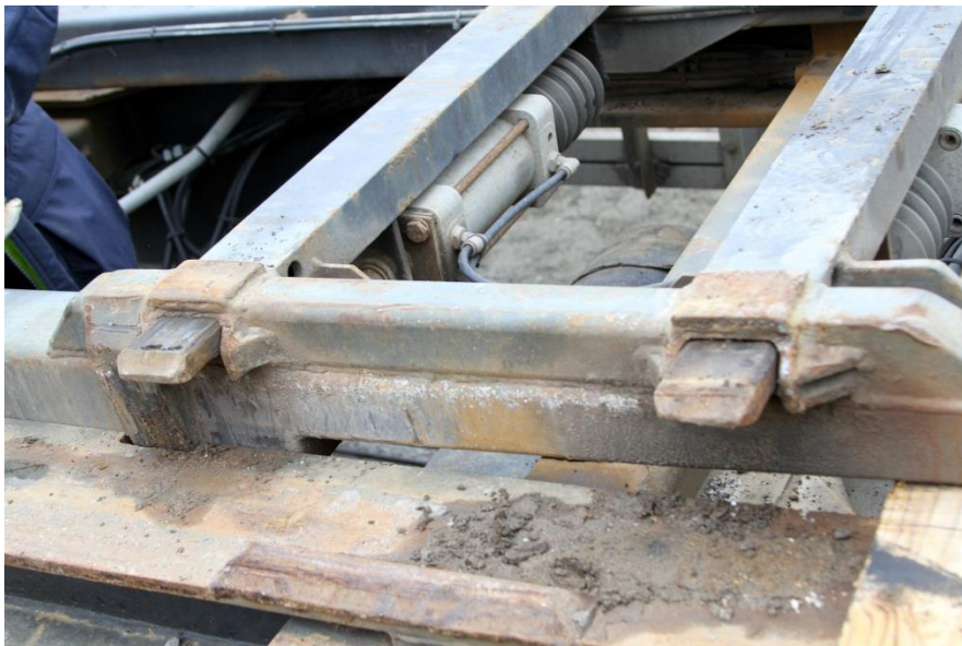
Photo 9. Securing device on the front part of the tilting frame
