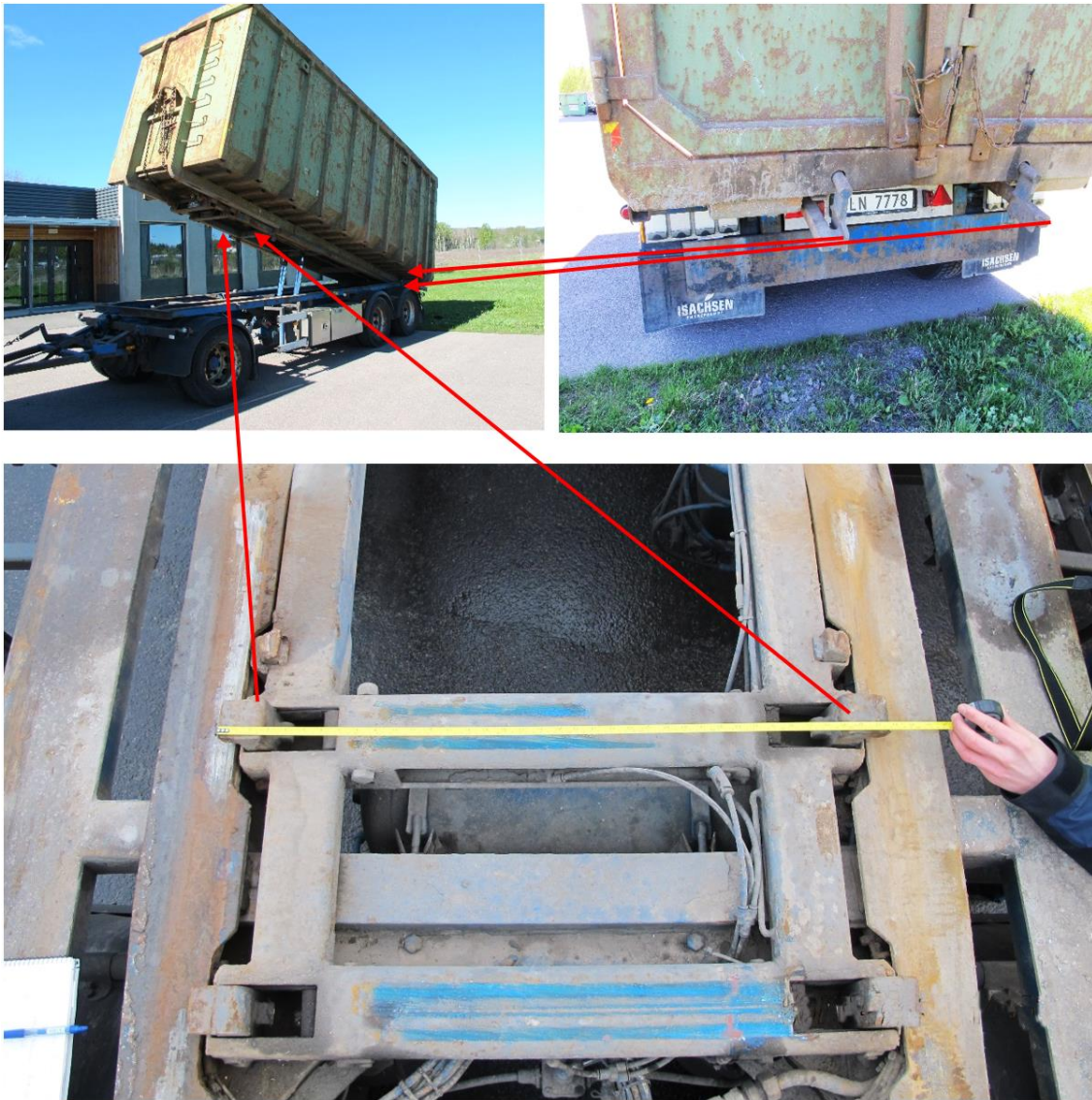
Figure 3: The container securing points: four pneumatic locking studs inside of the bottom side rails at the front and two stoppers at the rear. The rearmost locking studs were aligned to the recesses in the container's bottom rails at the time of the accident. The upper left photo shows an implemented measure whereby a chain is used between the container and tilt frame. Photo: AIBN
