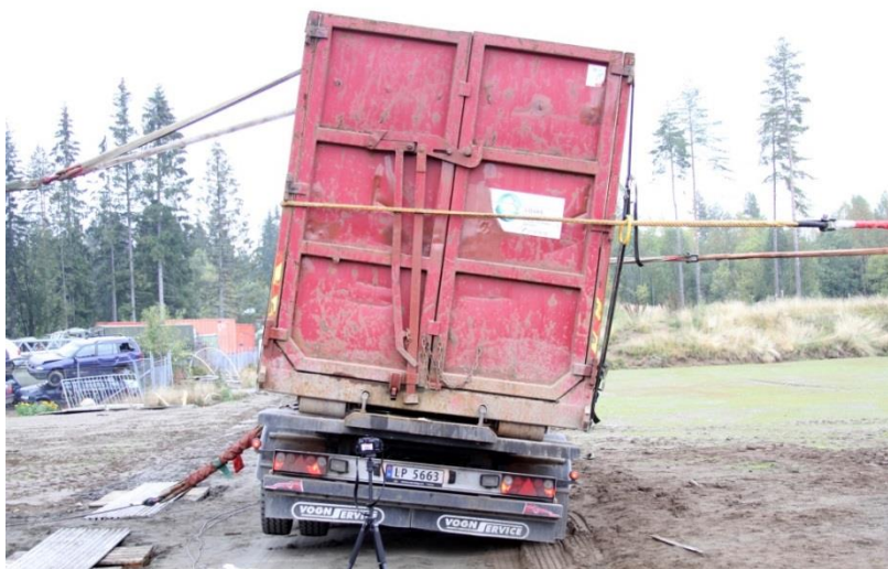
Photo 20. The wheels of the trailer lost contact with the ground at a force equivalent to an acceleration of 0,38g.
