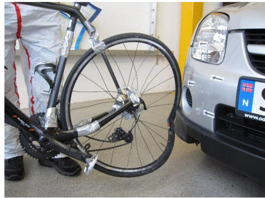
Figure 5: Assumed point of impact between the passenger car and the bicycle. Photo: AIBN
