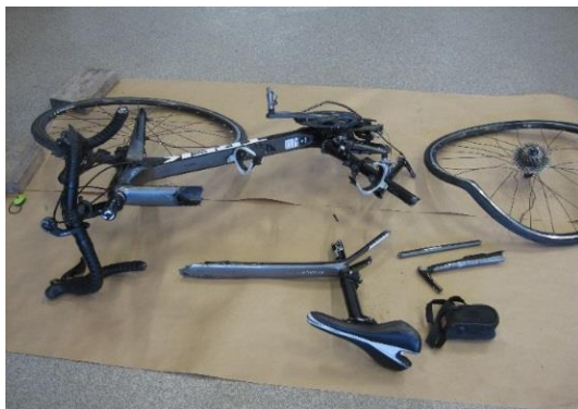
Figure 2: The bicycle frame broke into several parts, and the rear wheel was deformed. Photo: AIBN
