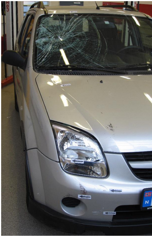
Figure 4: Damage to the right-hand side of the passenger car, with arrows marking the different dents/scratches/contact marks. Photo: AIBN
