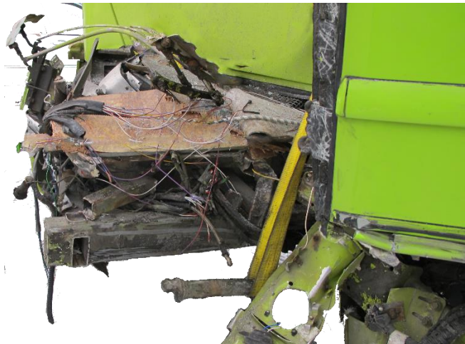
Figure 6: Cross-beam severed on the left-hand side, seen from the side. Photo: AIBN
