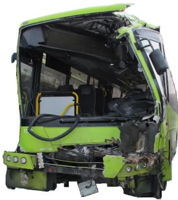
Figure 3: Damage to the front of the eastbound bus. Photo: AIBN
