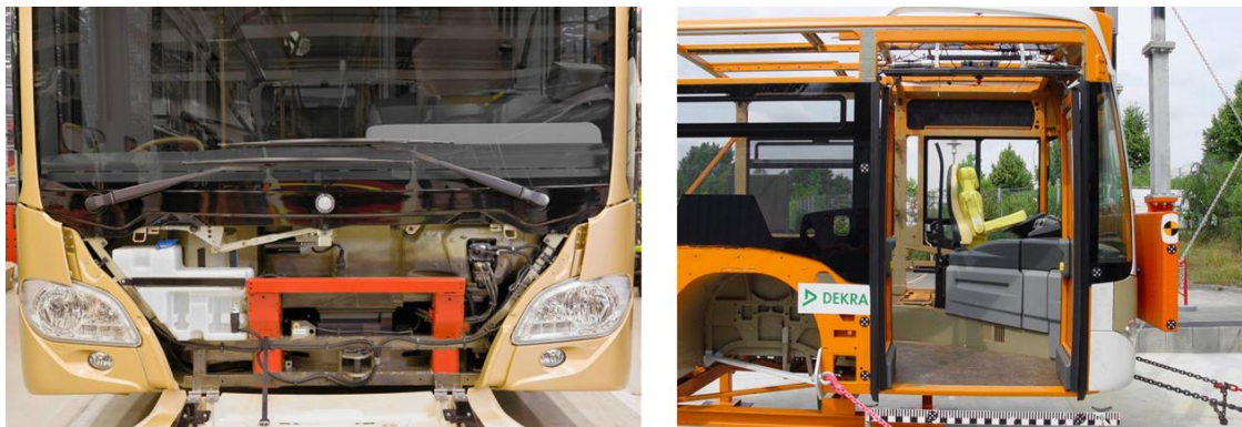
Figure 31: Reinforcement at the front of the Mercedes-Benz Citario, to comply with the requirements of UNECE-R-29. Photo: Mercedes-Benz, 2011
