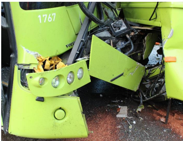
Figure 9: Overlap and penetration between the buses at the scene of the accident. Photo: NPRA
