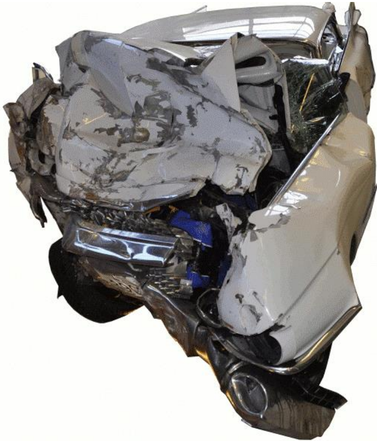
Figure 4: Deformation of the front of the accident car. Photo: AIBN
