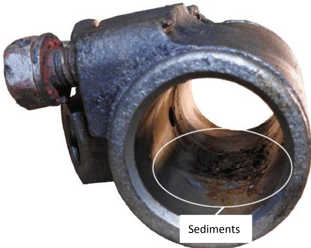
Figure 20: Piston housing, right front wheel cylinder. Photo and illustration: AIBN
