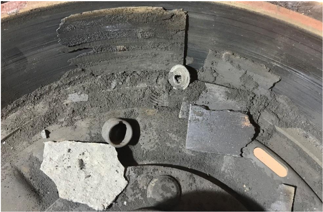
Figure 18: Parts of the brake band, brake dust and the hold-down spring inside the brake drum on the right front wheel. Photo: AIBN
