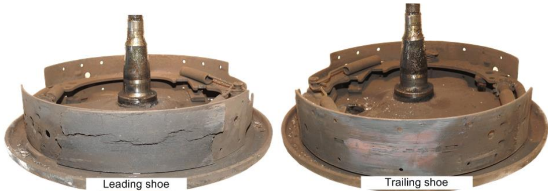
Figure 17: Brake band, right front wheel. The brake band on the trailing shoe was completely worn down. The brake band on the leading shoe was also worn. Photo: AIBN
