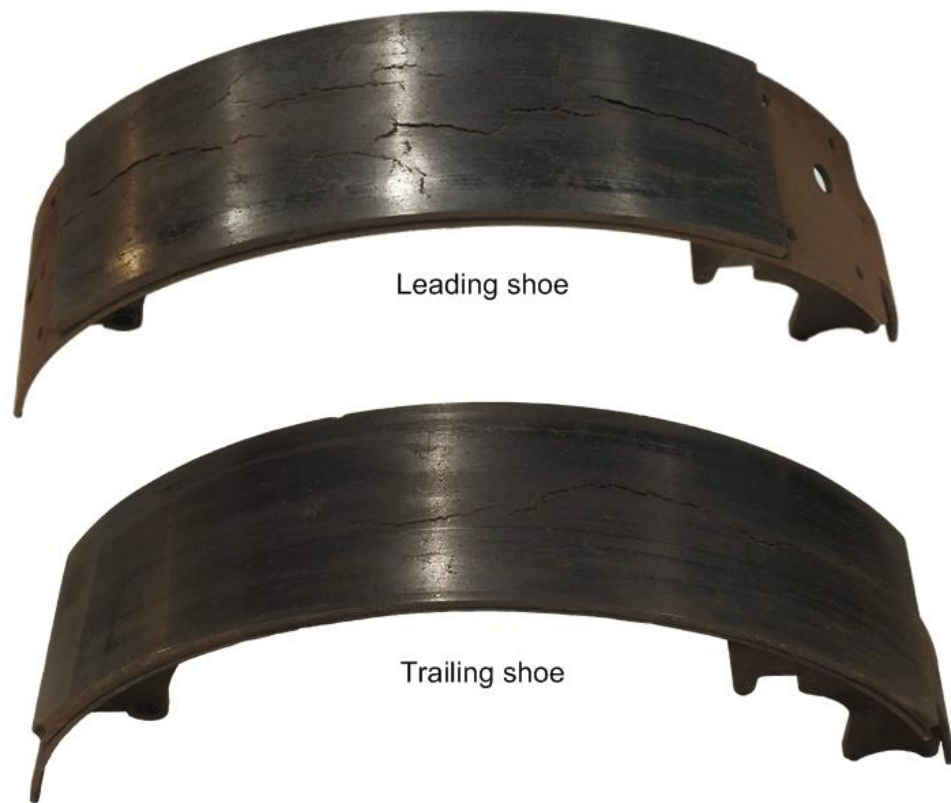
Figure 16: Brake shoe, left front wheel. Photo: AIBN
