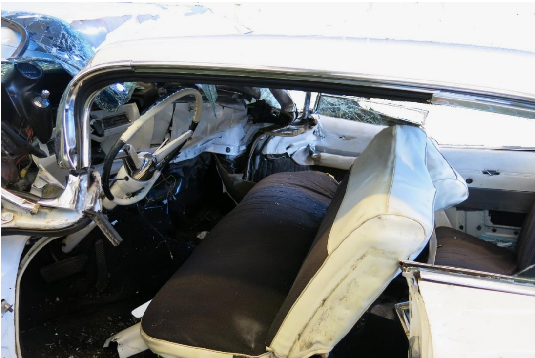
Figure 3: There was survival space in both the front and back of the car after the crash. Photo: AIBN
