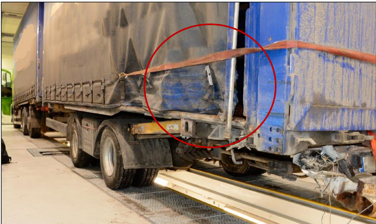
Figure 2: Damage to the left-hand side of the trailer. The red circle marks the point of impact with the passenger car. Photo: The NPRA
