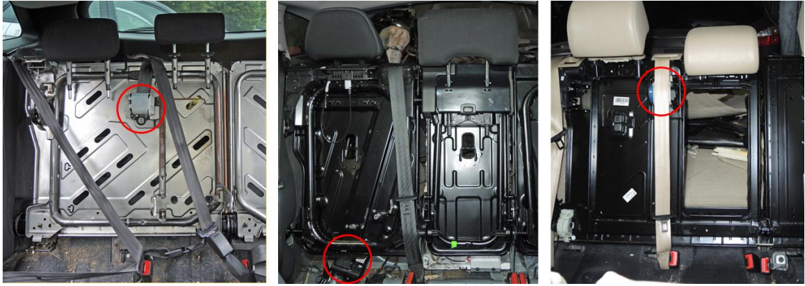
Figure 18: Design of seat belt integrated into rear seat-back for several manufacturers. The retractors are marked by red circles. Illustration: NSIA
