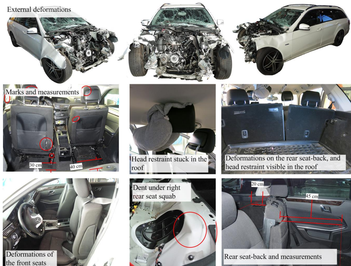
Figure 4: External/internal deformations, marks and points of impact in the estate car Illustration/photo: NSIA
