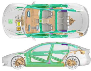
Figure 22: Tesla 3 (2018) has no pretensioners in the rear seat. Source: Euro Rescue
