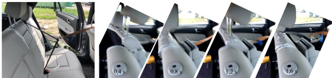
Pulling experiment, set-up Sequence of oscillations from the video (0,4 - 1,6 seconds)
