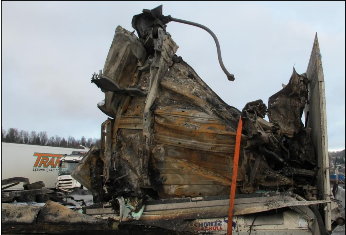
Figure 16: Fire damage to the driver's cab of the Norwegian tractor unit. Photo: NSIA
