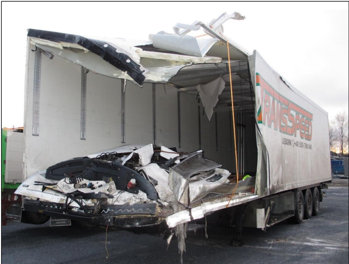
Figure 15: Damage to the Polish semi-trailer, which was carrying fish in polystyrene boxes. Photo: NSIA
