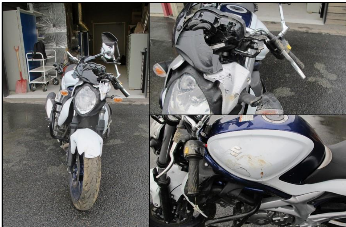
Figure 4: Damage to the motorcycle. Photo: NSIA
