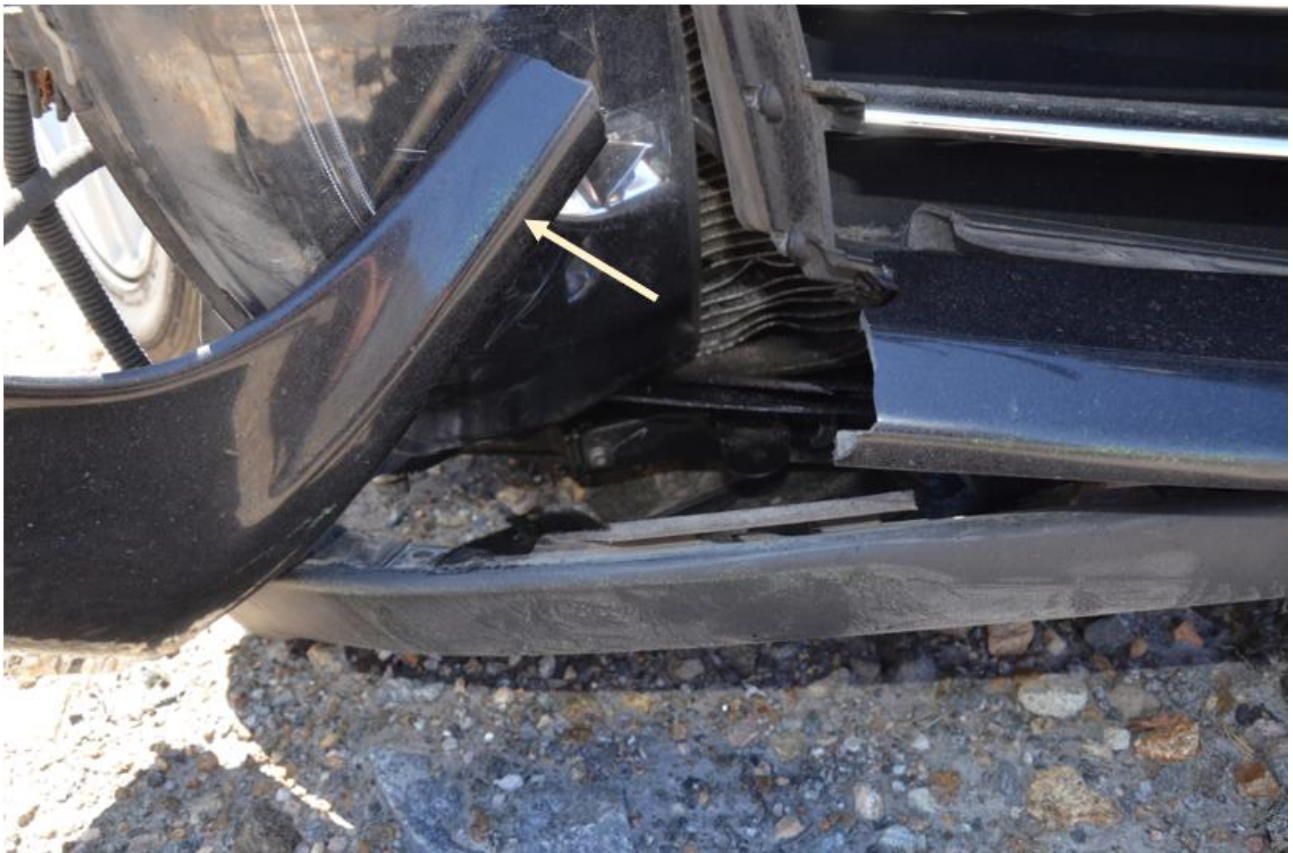
Figure 6: Lower part of the bumper and apron. The arrow indicates where traces of yellow textile were found. Photo: The police
