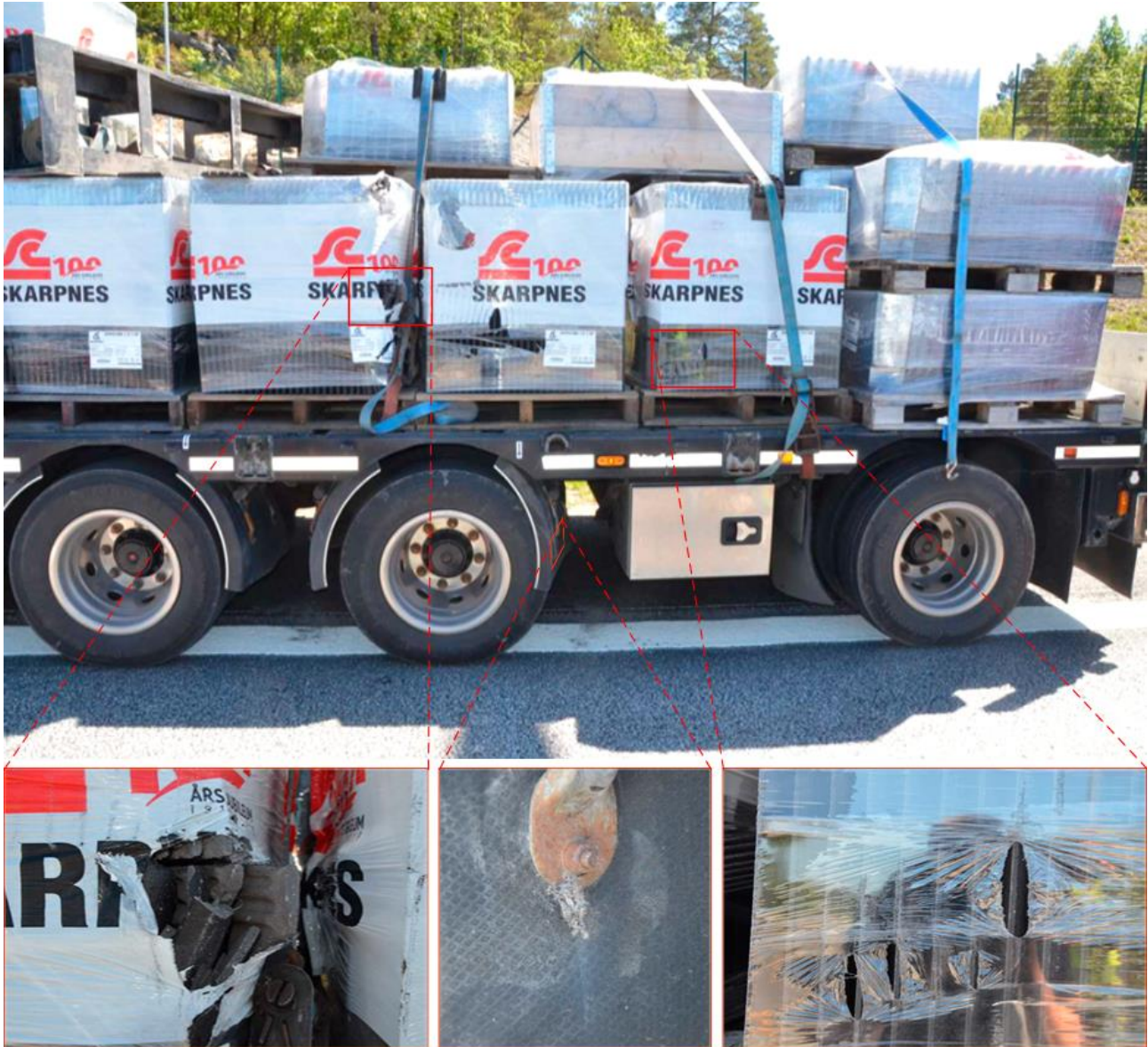
Figure 7: Damage to the cargo and packaging, and textile fibres found on the fender behind the left wheel on the semi-trailer's middle axle. Photo: The police. Illustration: NSIA
