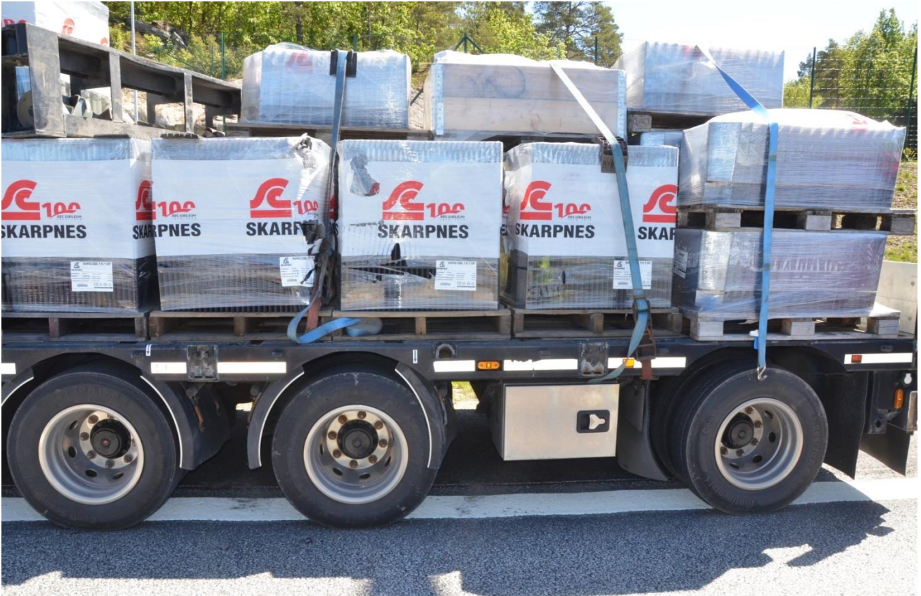
Figure 15: Location and securing of pallets on the semi-trailer. Photo: The police
