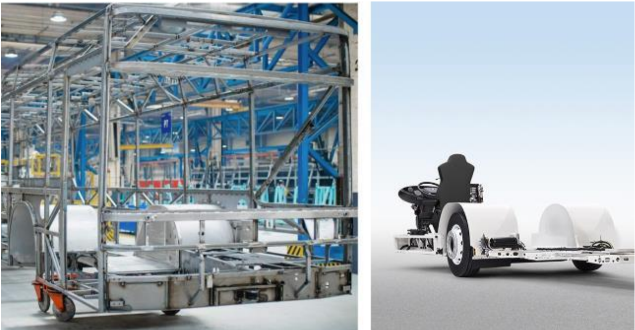
Figure 8: Bodywork and superstructure, and chassis on low-entry bus. Source: MAN.
