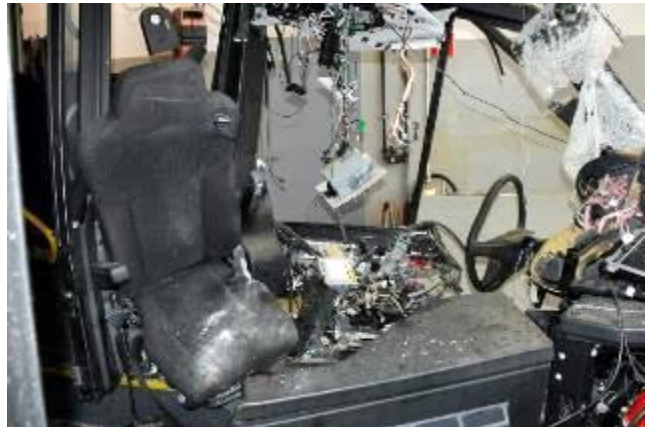
Figure 4: Driver's cab Bus 113. The driver's seat has been pushed backwards. Photo: NSIA
