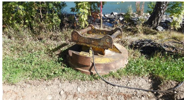
Figure 5: Excavator magnet used to collect bolts. Photo: NSIA
