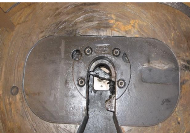
Figure 4: Crack formation and dent on the fifth wheel top plate, to the right of the locking mechanism. Photo: NSIA
