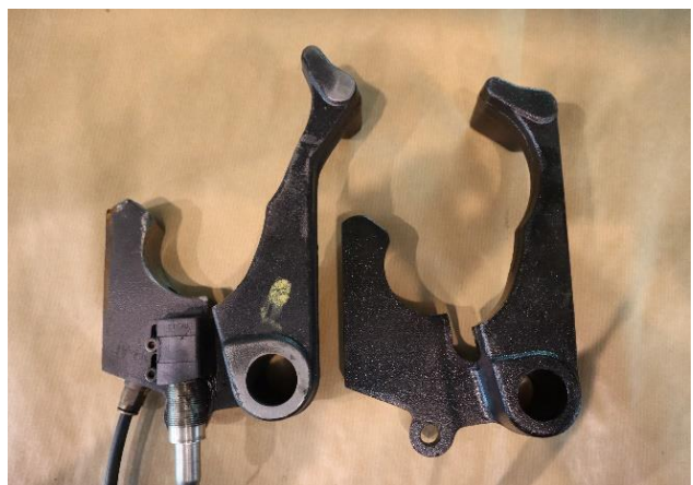
Figure 5: Lock jaw, damaged example on the left, new on the right. Photo: NSIA
