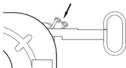
Figure 5 - Locking of a fifth wheel with a Standard handle
