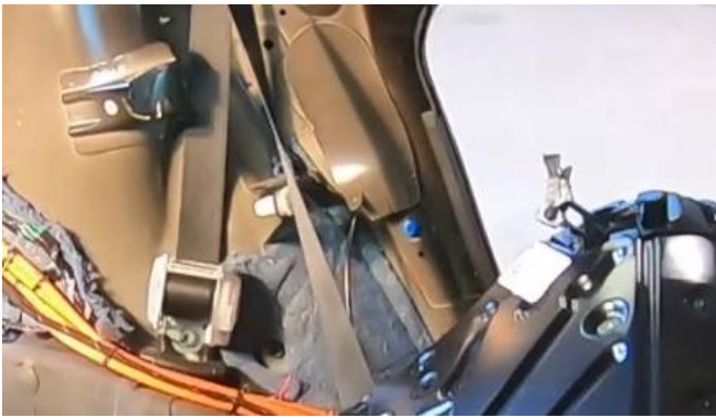
Figure 36: Torn-off striker and loop left hanging in the rear seat-back. Photo: NSIA
