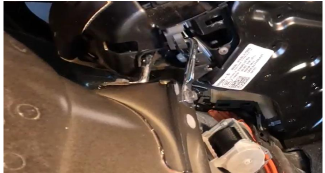
Figure 34: Test #2 distortion and contact between latch and striker loop at 740 kg. Source: NSIA
