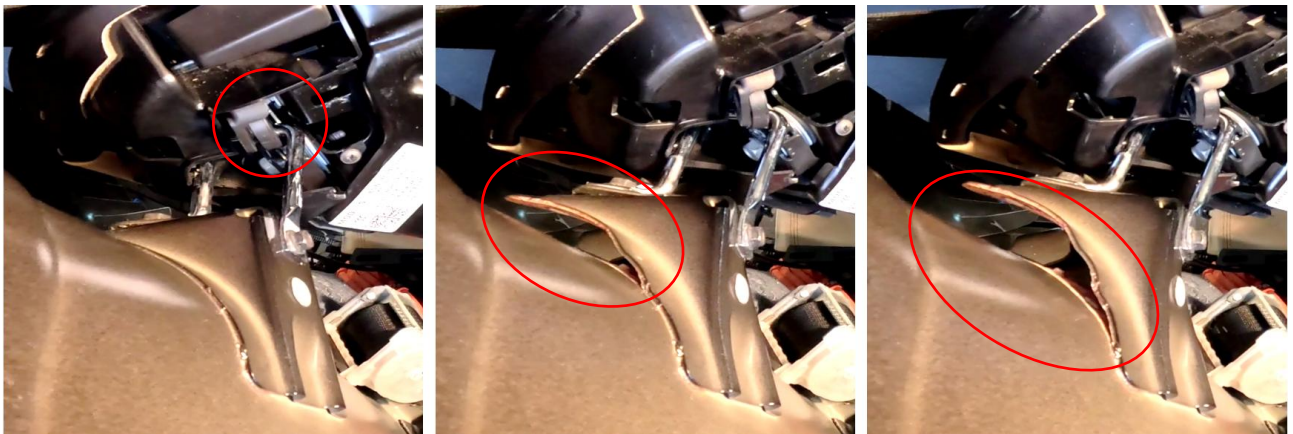
Figure 35: Sequence from test #2. Distortion of the rear seat-back as a result of tension led to the latch in the rear seat-back coming near the corner of the striker loop. There was lateral tension on the striker via the loop and the rear seat-back's striker to the wheel arch was torn clean off. Screenshot: NSIA
