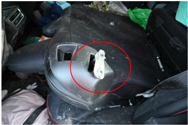
Figure 8: Torn-off striker that lodged in the lock of the rear seat-back (60-part). Photo: Norwegian Public Roads Administration
