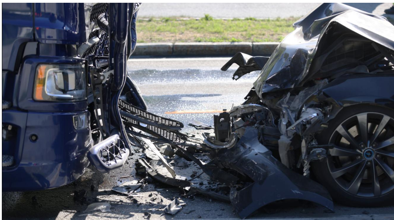
Figure 5: Deformation of the tractor unit and passenger car after the collision. Photo: Tangen foto
