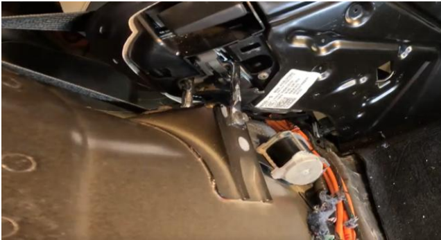
Figure 33: Test #1 distortion just before the shoulder belt broke at 1,660 kg. Source: NSIA
