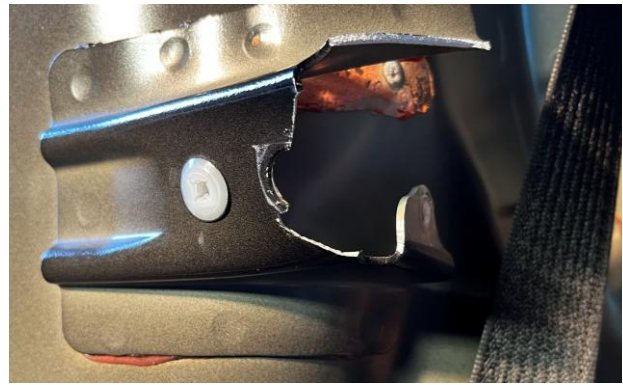
Figure 37: Torn-off striker beside the wheel arch. Photo: NSIA
