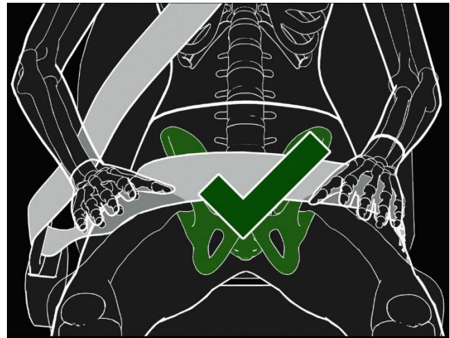
Figure 47: Correct positioning of the lap section of the seat belt. Illustration: NSIA
