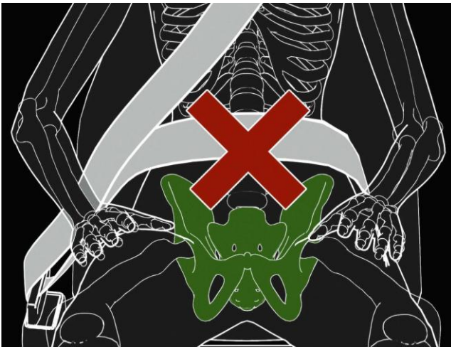
Figure 46: Incorrect positioning of the lap section of the seat belt. Illustration: NSIA
