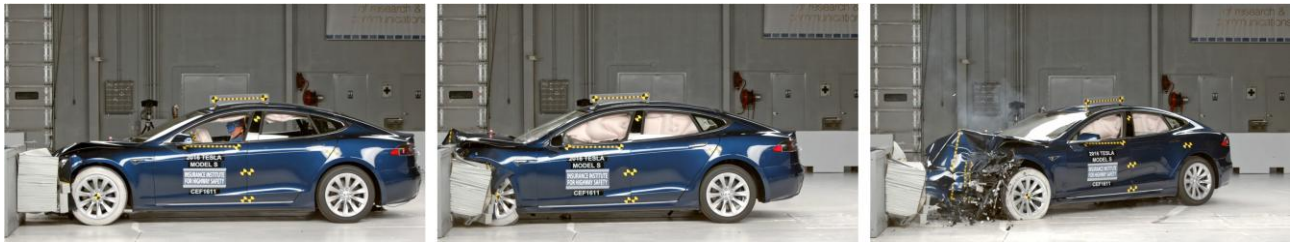
Figure 45: Tesla model S 2016 during crash test with moderate overlap at 64.4 km/h. Source: IIHS, CEF1611, FLO03_WIDE
