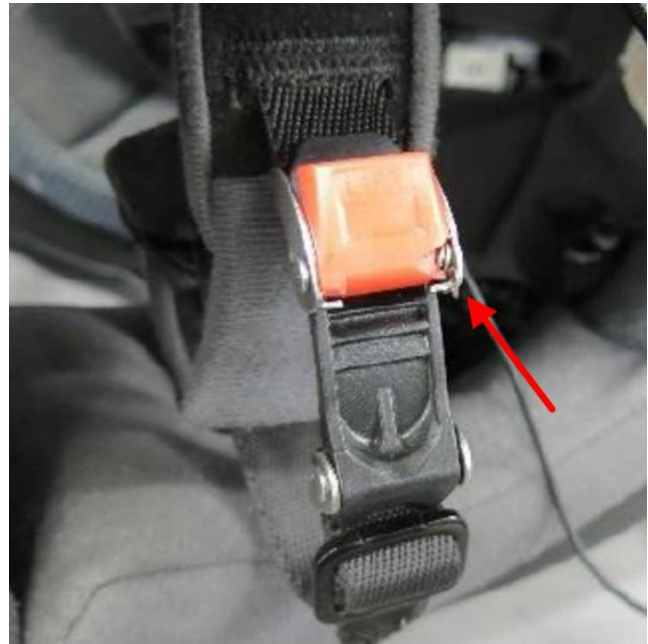
Figure 2: Damaged fastening mechanism (quick release) on the motorcyclist's helmet on county road FV 115 in Indre Østfold. Photo: The Research Institute of Sweden (RISE).
