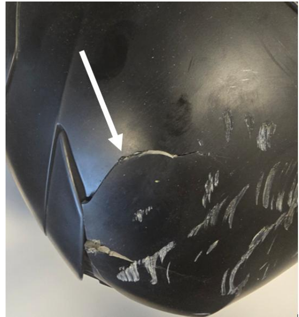
Figure 6: Crack (white arrow) in the rider's helmet from the E10 accident in Tjeldsund. Photo and labelling: NSIA
