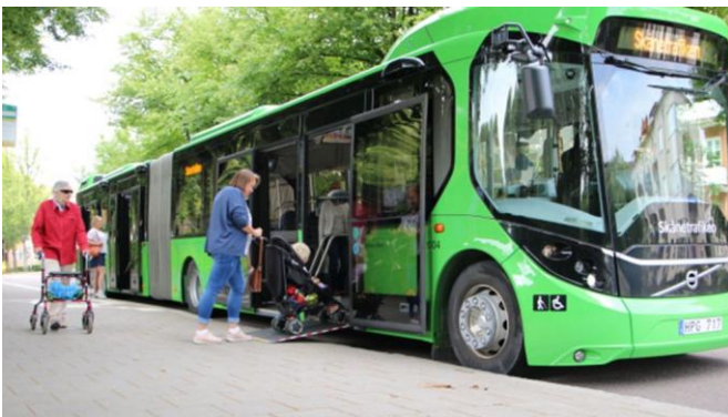
Figure 26: Volvo concept bus 2016. Central driving position and forward passenger entrance behind the front axle. Photo: Volvo bus
