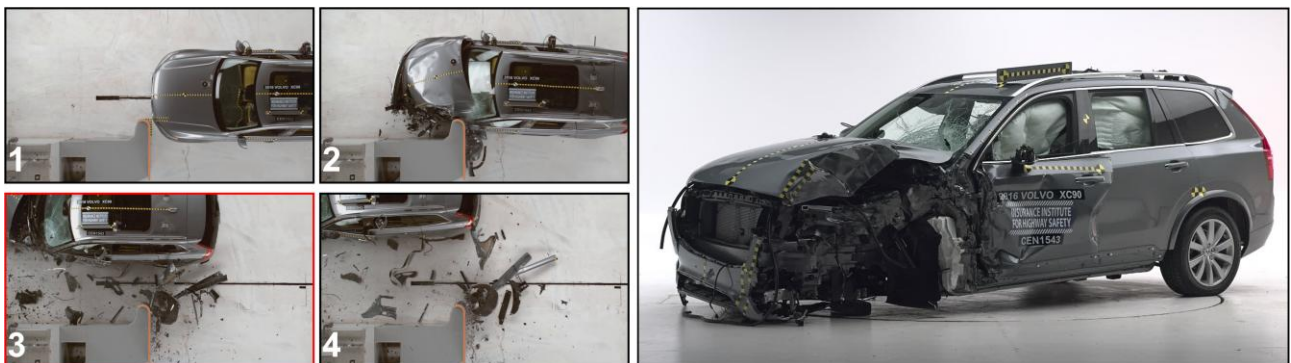
Figure 18: Test of a 2016 Volvo XC90 ( CEN1543 ) Small Overlap Front Test, sequences 1–4, and damage post-test. Source: IIHS
