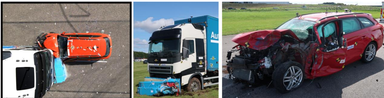
Figure 29: Collision trial and vehicle damage with an energy-absorbing front structure in the form of a solid plate installed on the heavy goods vehicle. Each vehicle had an impact speed of 50 km/h in the tests. Photo: Swedish Transport Administration/Chalmers
