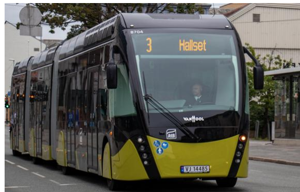
Figure 27: Van Hool ExquiCity i Trondheim. Almost central driving position and forward passenger entrance behind the front axle. Photo: AtB AS
