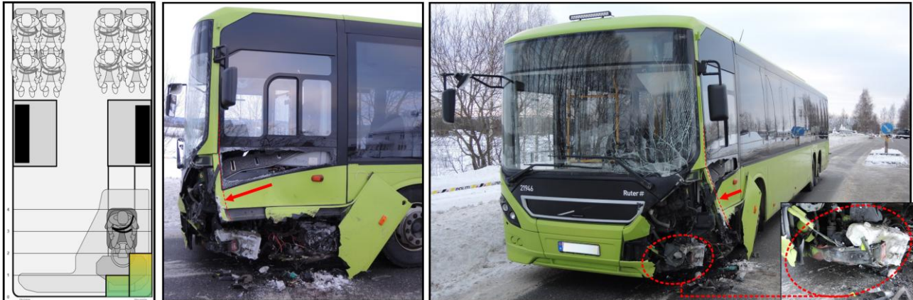
Figure 20: Vehicle damage illustrated on the left. The bent front crossmember and outward twisting of the left sidewall are marked. Photo, markings and illustration: NSIA
