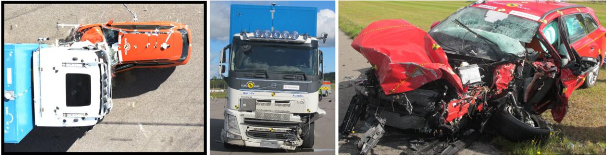
Figure 28: Crash test and vehicle damage with a rigid front on the heavy goods vehicle. Each vehicle had an impact speed of 50 km/h in the tests. Photo: Swedish Transport Administration/Chalmers
