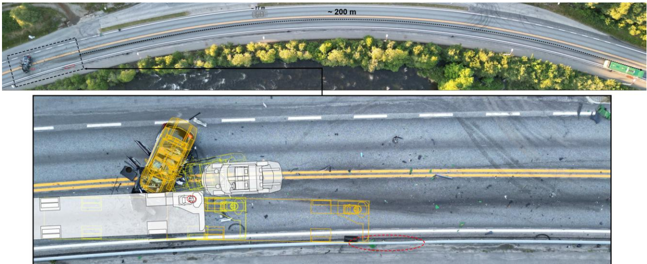
Figure 13: Overview of the accident site, estimated point of impact, and vehicle movement immediately following the collision. Photo: Norwegian Public Roads Administration. Illustration: NSIA
