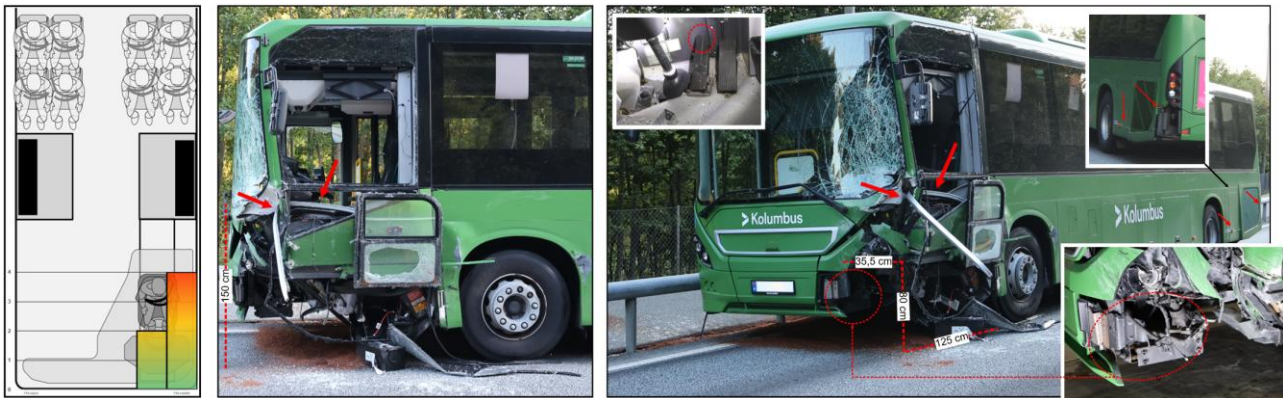
Figure 14: Vehicle damage illustrated on the left. Images of the jammed brake pedal, the area around the bus's front left crossmember, and scrape marks extending rearwards along the left-hand-side of the bus. Photo: Norwegian Public Roads Administration. Markings and illustration: NSIA
