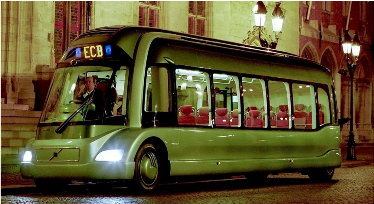
Figure 25: Volvo ECB 1995, a bus with 30 seats and a central driving position. Photo wiki.gearknob.org
