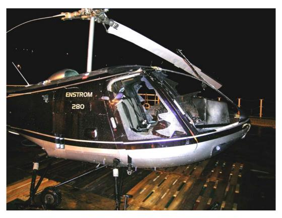
Figure 4: The helicopter photographed at night after it had been salvaged. The front windscreen and the windows in both doors are shattered. Further, the damage on the front and the bending of the main rotor blades are visible.
