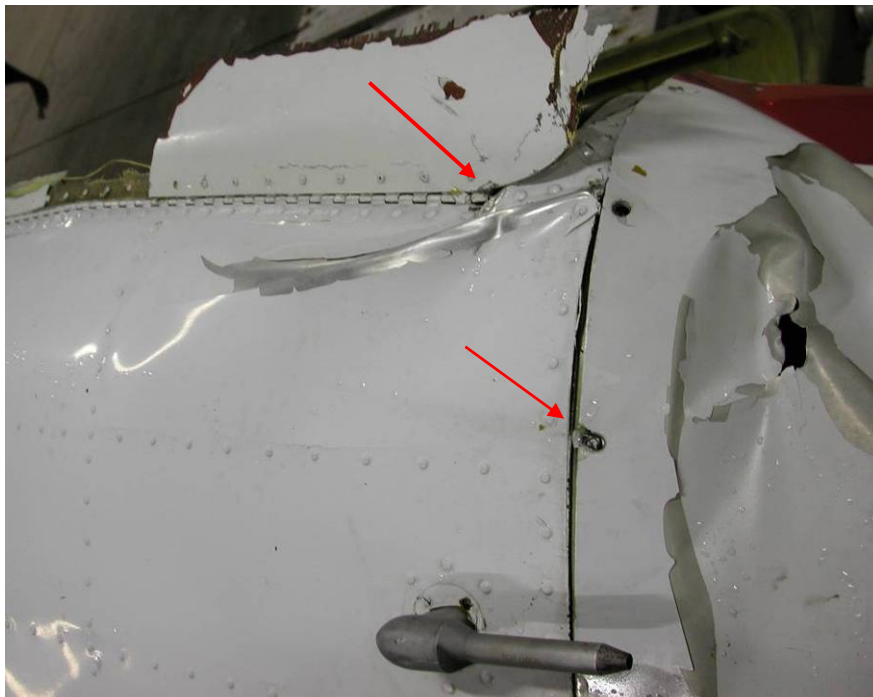
Figure 11: Photo of the aircraft's nose. Front of the aircraft is to the right. The red arrows show the impact points.
