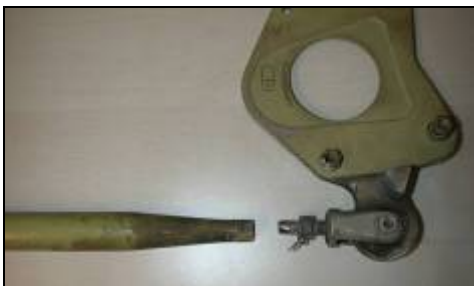
Figure 7: Broken elevator transfer rod
