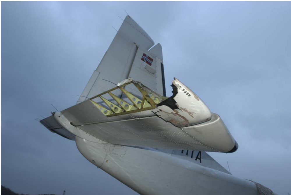
Figure 6: Damage to the right elevator (photo taken by armed forces)
