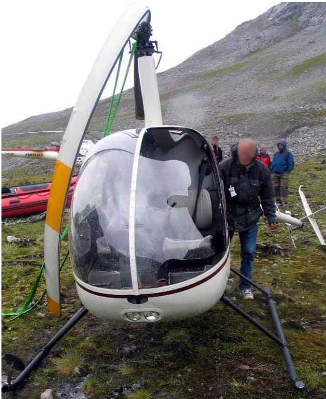
Figur 13: Frontvindu venstre side (frontvindu er knust.)
