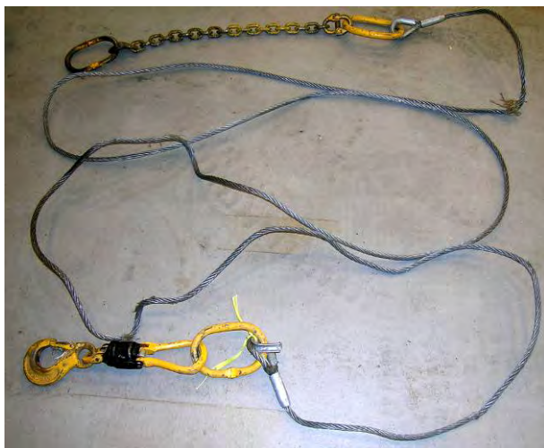
Figur 13: Lastewiren "Wire Sling".
