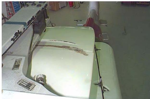
Image 4. Blade Bolt-Cowling Contact
