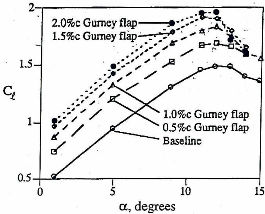
FIGUR 3 - Data for NACA 4412 vingeprofil m/ Gurney flap
