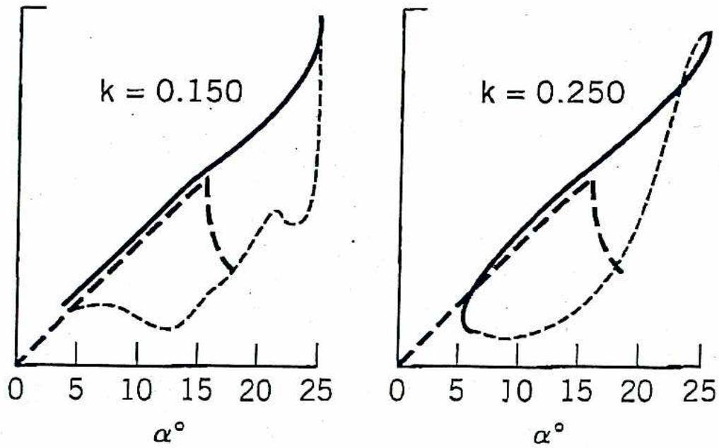
FIGUR 4 - Hysteresis for NACA 0012 vingeprofil
