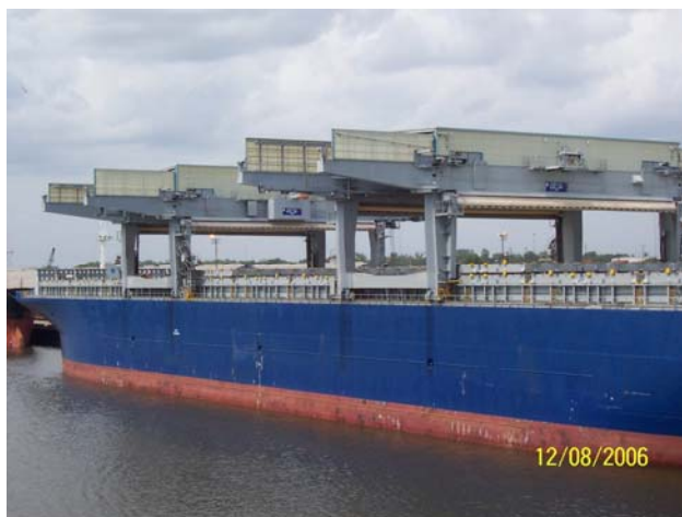
Figure 3: Gantry cranes (the photo is from Star Isfjord ).
