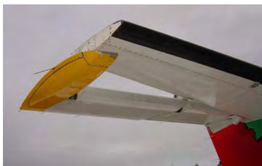
Fig. 1 OY-JRJ's elevator seen after landing
