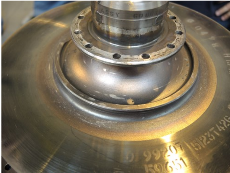
Aft flange of the centrifugal Impeller. Photo: NSIA
