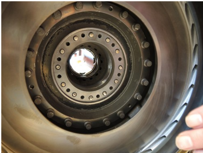
Forward flange of the turbine shaft. Photo: NSIA
