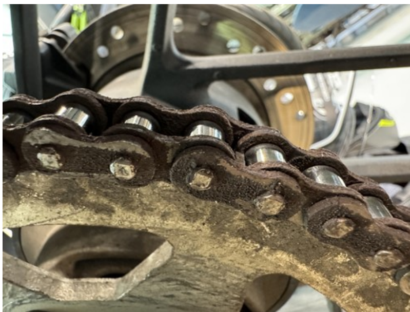
Wear and insufficient maintenance of chain. Photo: NSIA
