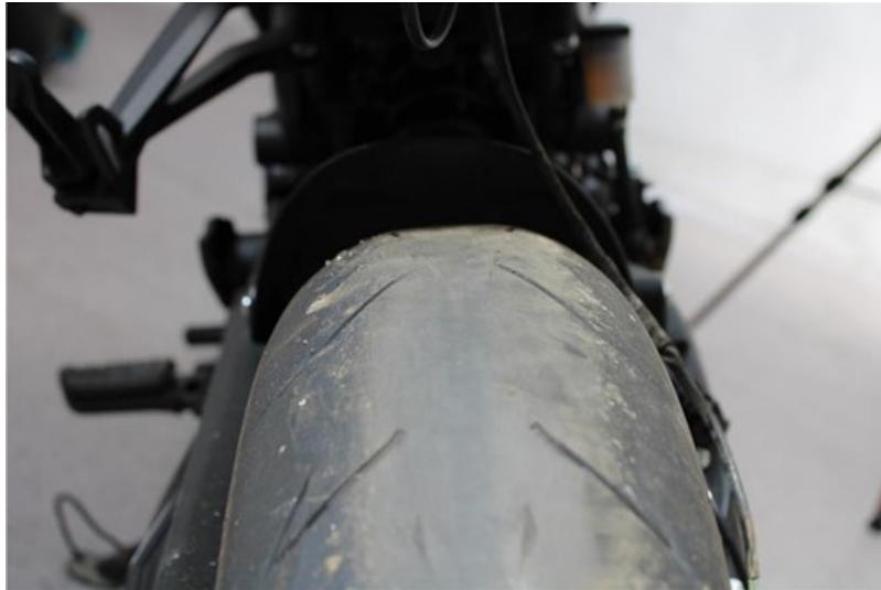
Insufficient tread depth on tire. Photo: NSIA
